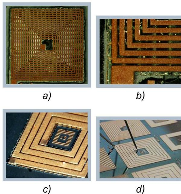
Figure 4. Half-permalloy inductors. a) and b) show a 19-turn inductor, c) shows the four-turn inductor characterized, and d) shows an inductor undergoing component-level characterization with a HP 4194A impedance analyzer. gap and presents a more severe topology over which the top NiFe layer must be electrodeposited.
