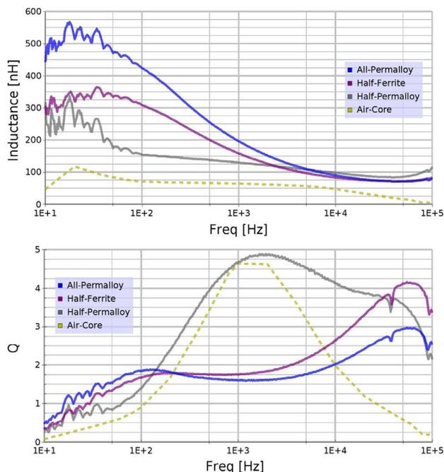
Figure 6. Component-level characterization results. Not surprisingly, the all-permalloy inductor shows the largest inductance. It is believed that eddy currents lower the Q for the all-permalloy inductor, but B-H hysteresis losses lower the half-ferrite inductor's Q. Note that around 10 MHz, the half-ferrite inductor has approximately the same inductance as the half-permalloy, but a lower Q.
