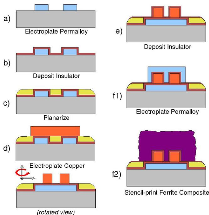
Figure 3. Fabrication process for inductors. Step d) represents a completed half-permalloy inductor, while steps f1) and f2), respectively, represent completed all-permalloy and half-ferrite inductors.
