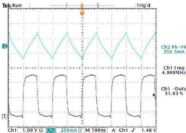
Figure 8. Waveforms showing operation of prototype DC/DC converter. The top trace (200 mA/div) is inductor current. The bottom trace (1 V/div) is the switched output voltage, taken at the node joining the inductor and the DC/DC IC's output transistors.
