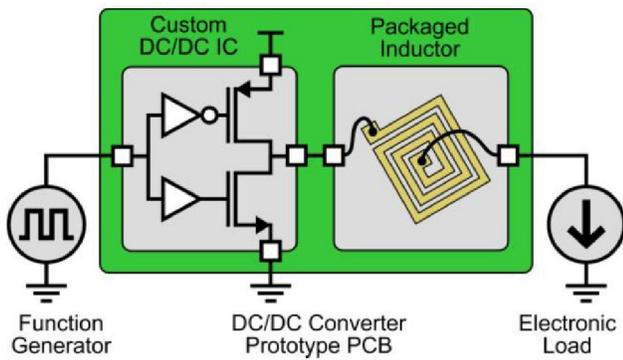
Figure 7. In-system characterization schematic. Though the system was packaged as a PCB, the DC/DC IC was built using typical CMOS technology, and is thus representative of the circuitry that would be used in a practical integrated converter.
