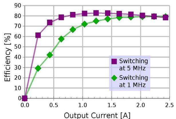
Figure 9. In-system characterization results. The lower-amplitude AC current at the faster switching frequency is credited with the increase in efficiency
