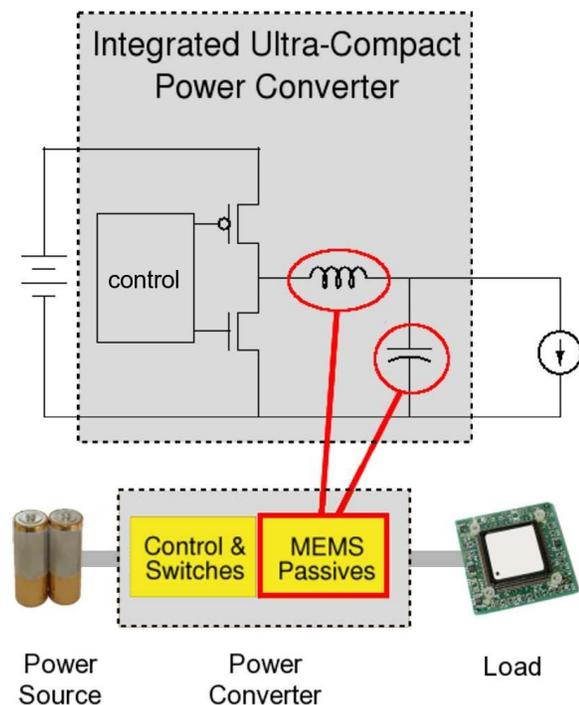
Figure 1. Schematic illustration of electronic system incorporating power conversion for voltage supply. The highlighted components would be integrated into a single silicon die to produce an ultra-compact power converter.
