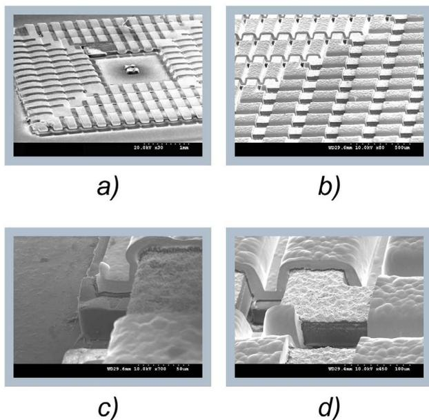
Figure 5. SEM Images of all-permalloy inductor. Due to a smaller gap between copper lines, the inductor pictured in a) exhibits better planarization between the copper and top NiFe layers. In contrast, the inductor in b), c), and d) has a much larger gap.
