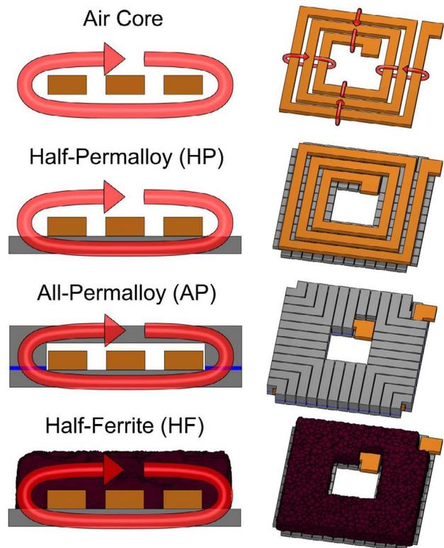
Figure 2. Cross-section and perspective views of the four investigated core constructions. In all diagrams, the translucent red arrow represents the magnetic field produced by current in the coil.
