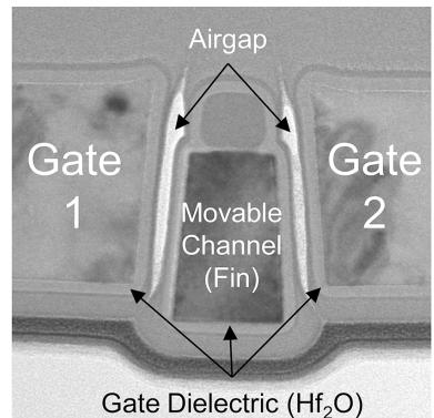
Figure 4: Cross section image of Fin-FACT by use of TEM. Airgap and thickness of gate dielectric is 50 nm and 30 nm, respectively.
