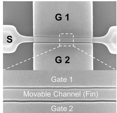
Figure 3: Top-view image of fabricated Fin-FACT using SEM. The magnified SEM image is also obtained for verification of thickness of movable Si-channel.
