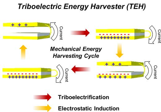
Figure 2: Operation principle of a triboelectric energy harvester (TEH). TEH shows several features. Particularly, TEH generates higher output voltage than any other energy harvesting methods.
