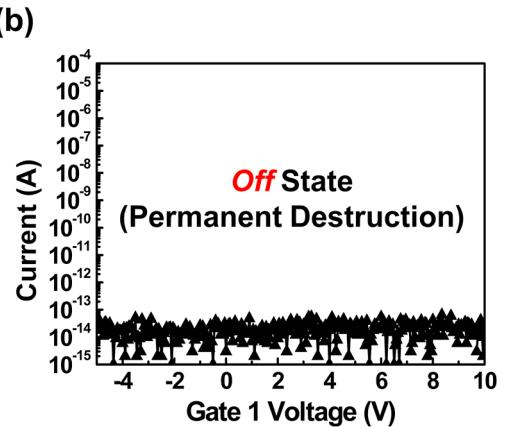
Figure 7: Electrical characteristics of NEM switch in two states. (a) Drain current according to gate voltage for switch turn-on. (b) Drain current according to gate voltage for destruction of movable fin channel.
