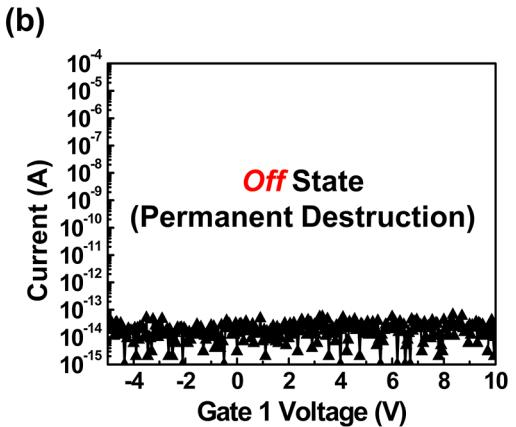
Figure 7: Electrical characteristics of NEM switch in two states. (a) Drain current according to gate voltage for switch turn-on. (b) Drain current according to gate voltage for destruction of movable fin channel.
