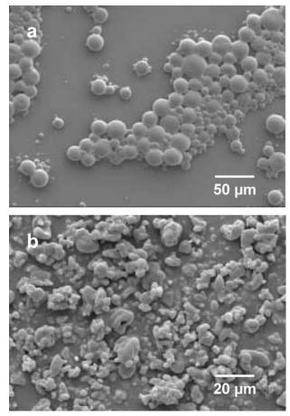
**Fig 4** Microparticles used for particle-based micromolding imaged by scanning electron microscopy. (a) PLA microparticles prepared by a double-emulsion technique. (b) PLGA 50/50 microparticles prepared by spray drying
