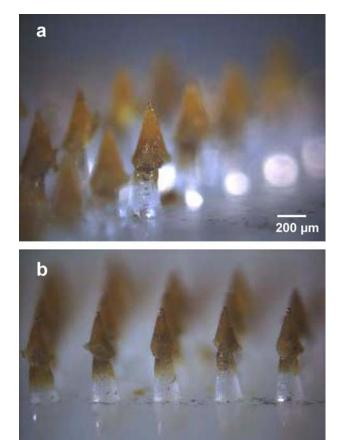
Fig. 9 Microstructures with complex arrowhead geometry. A portion of an array of 200 microneedles is shown at two different magnifications. The yellow/brown arrowheads are made of PLGA encapsulating Vitamin B and the transparent shafts are made of PLA. Each microneedle has a 250  $\mu$ m base diameter and a 750  $\mu$ m height (a) side view (b) front view
