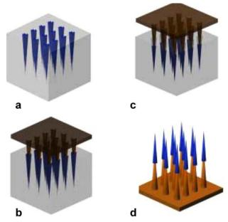
Fig. 3 Fabrication of microstructures with complex arrowhead geometry. (a) Polymer microparticles are filled into a mold and residual particles are removed from the surface. A microstructure previously prepared out of a polymer with a higher melting point using the same mold is aligned and inserted part way into the mold. (c) The microparticles are melted. (d) The resulting microstructure with a complex arrowhead geometry is removed from the mold
