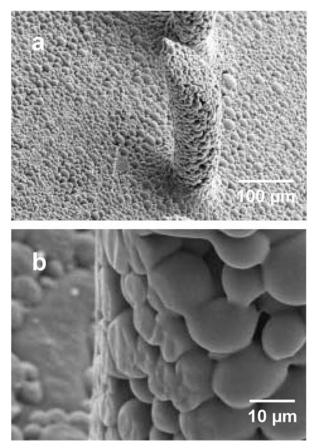
**Fig 5** Porous microstructure fabricated by ultrasonic welding imaged by scanning electron microscopy. (a) A portion of an array of porous, beveled microneedles measuring 600  $\mu$ m in height and 100  $\mu$ m in base diameter. (b) A magnified view showing the individual PLA microparticles welded together to form the microstructure
