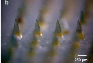
Fig. 6 Microstructures layered with multiple materials viewed by brightfield microscopy. (a, b) A portion of an array of 200 microneedles is shown at two different magnifications. The transparent green tips are made of PLGA encapsulating green dye and the opaque yellow shafts are made of PEG containing PLGA particles encapsulating Vitamin B. Each multi-layered microneedle has a base length of 250  $\mu$ m, a tip length of 5  $\mu$ m, and a height of 600  $\mu$ m
