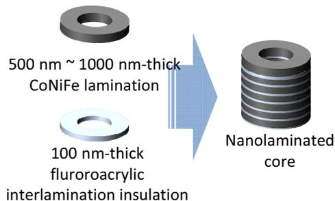
Figure 1. Schematic of a nanolaminated core.
