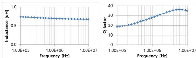
Figure 6. Inductance (Left) and Q factor (Right) of a microfabricated inductor with directly-patterned windings.
