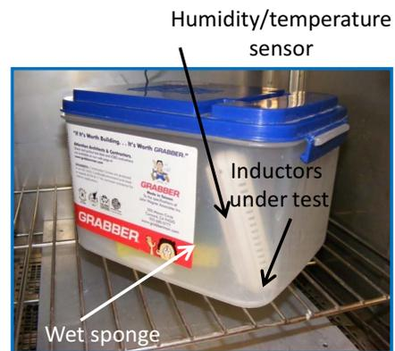
Figure 9. Corrosion test setup.
