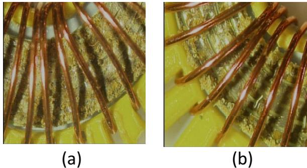
Figure 11. Optical microscope images of an (a) SU-8 anchor core and a (b) self-assembled core after 90 days of corrosion test.
