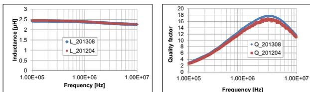
Figure 8. Inductance (Left) and Q factor (Right) of a device after 16 months at ambient conditions (L\_201308, Q\_201308).
