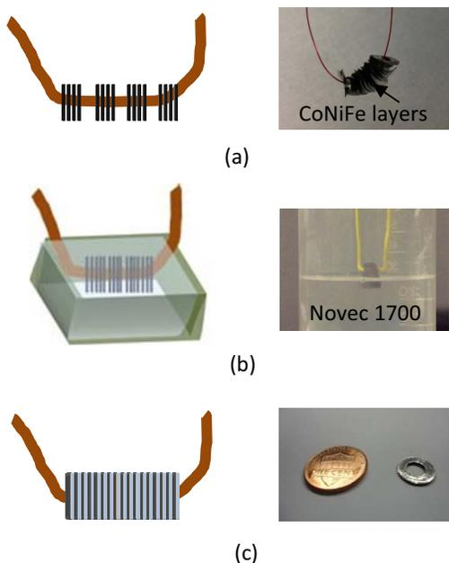
Figure 2. Fabrication of a nanolaminated core based on surface tension-driven assembly.
