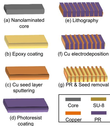
Figure 4. Microfabrication of a coil based on direct patterning method.
