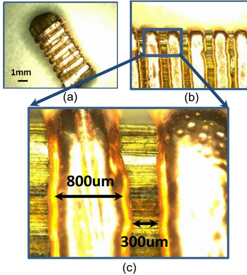
Figure 5. (a) Low magnification, (b),(c) high magnification optical images of the nanolaminated core wound by directly-patterned coils.
