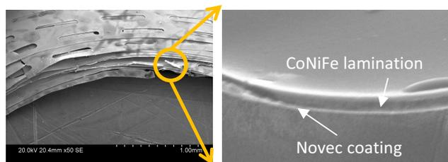
Figure 3. Scanning electron microscope image of a nanolaminated core. The core is manually cross-sectioned to observe Novec coating (Left). The magnified view of the cross-section of a single magnetic layer (Right).
