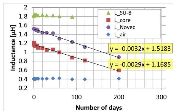
Figure 10. Measured inductances of the devices (at 3 MHz) throughout 200 days in the corrosion chamber.
