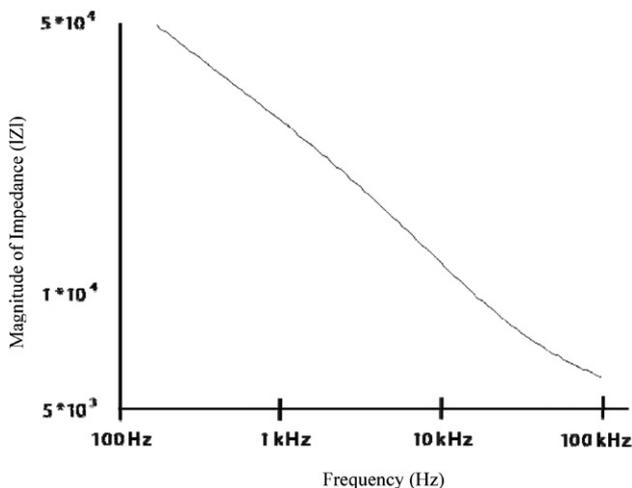
**Figure 9.** Magnitude of the electrical impedance of tweezers with an embedded platinum-black electroplated microelectrode.
