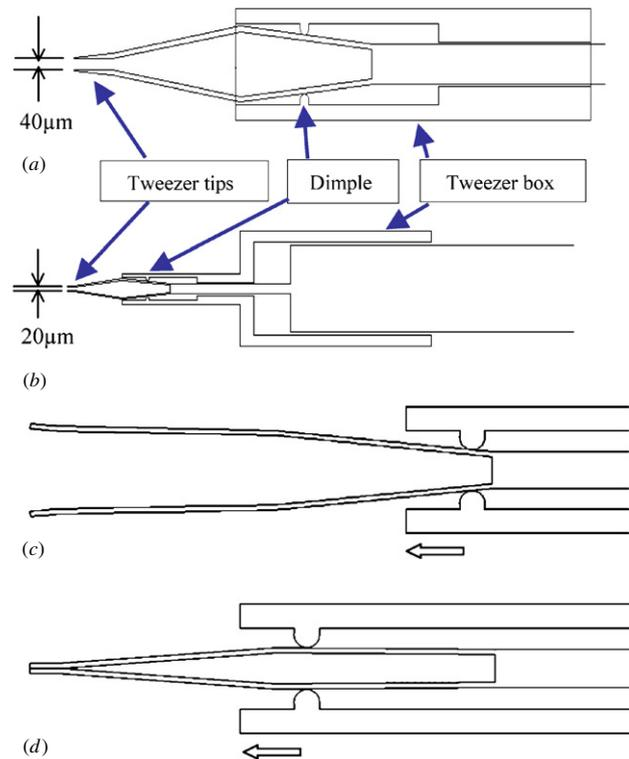
**Figure 1.** Design of mechanical microtweezers. (a) Gap of the tip: 40  $\mu\text{m}$ , width of the tip: 20  $\mu\text{m}$ . (b) Gap of the tip: 20  $\mu\text{m}$ , width of the tip: 10  $\mu\text{m}$ . (c) Open state of the microtweezers. (d) Closed state of the microtweezers.
