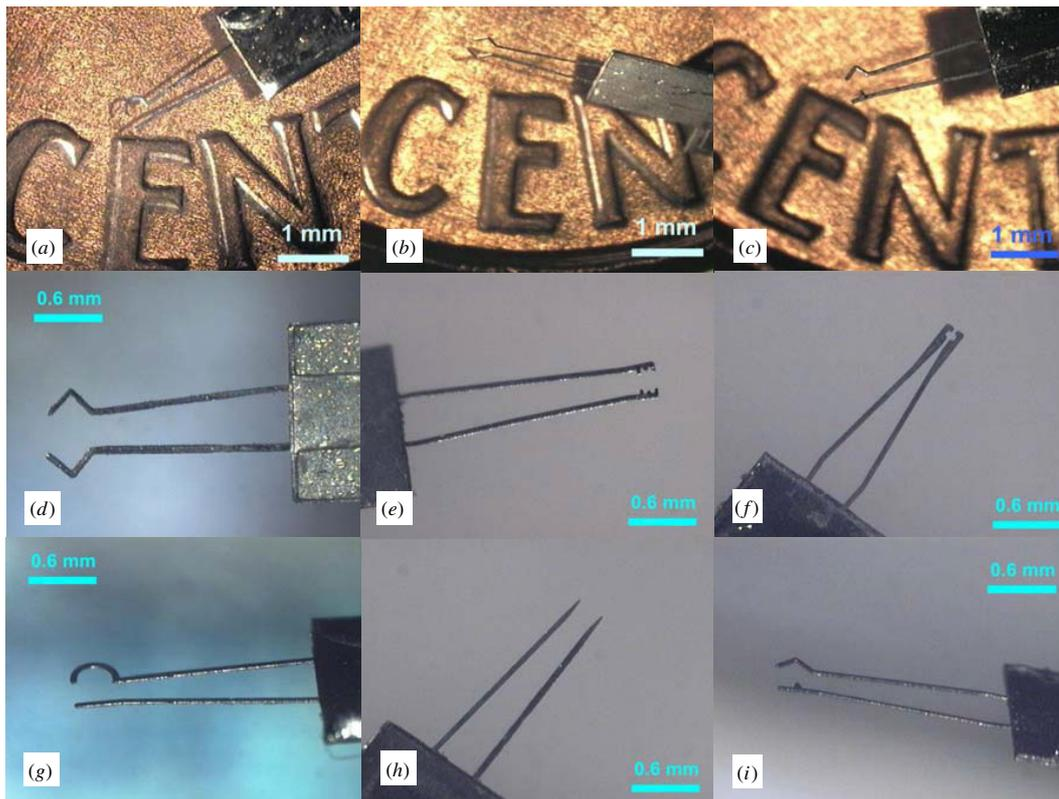
**Figure 7.** Various designs of the microtweezer tip. (a) Scoop, (b) diamond, (c) piercing, (d) diamond, (e) multi-prong, (f) circle-notch, (g) scoop, (h) sharp and (i) piercing.
