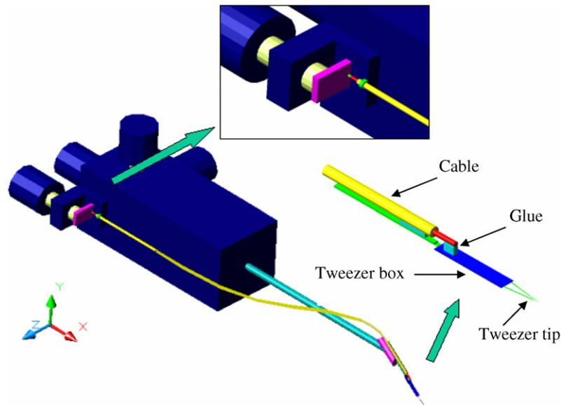
**Figure 2.** 3-D view demonstrating the fundamental principle of operation. An axis knob on a microprobe station controls the motion of the tweezer box through a tethered cable.
