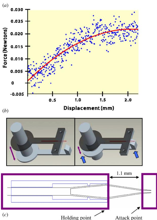
**Figure 6.** (a) Force curve of a tweezer electrode demonstrating the mechanical strength of the tweezer tip beam over a vertical displacement test. (b) Schematic view of the test setup using an Instron MINI55 materials testing system. (c) Two points for the force test. Force levels out 0.02 N after the tweezer tip is permanently deformed.
