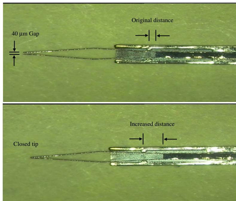
**Figure 4.** Demonstration of the actuation mechanism using a tweezer box with removed top. Open and closed states of the microtweezers is shown. For this particular tweezer model, the tip separation is 40 μm and the width of the tweezer tip beams are 20 μm.
