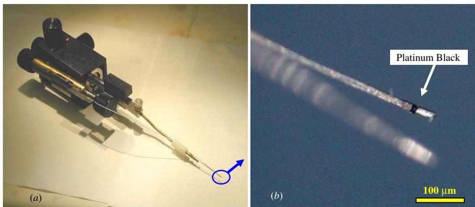
**Figure 8.** (a) Microtweezers are fastened to a micromanipulator with an attached, additional control knob for tweezer actuation. (b) The magnified view of the tweezer tip. Tip is coated with parylene and platinum black is electroplated on a microelectrode for electrophysiological stimulation and recording of neural systems.
