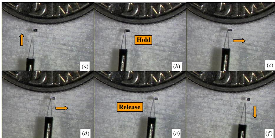
**Figure 5.** Pick and place operations to show the functionality of the microtweezers. A small piece of 10  $\mu\text{m}$  thick film is used as a target object.
