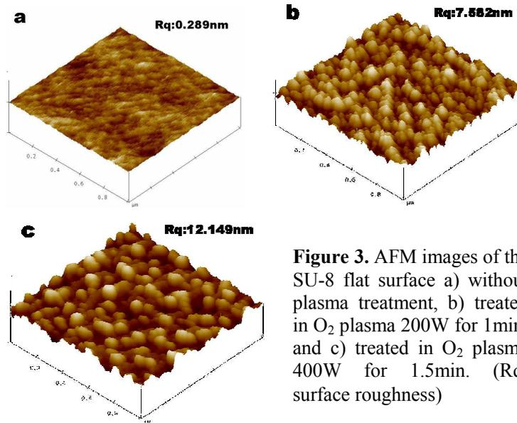
**Figure 3.** AFM images of the SU-8 flat surface a) without plasma treatment, b) treated in O<sub>2</sub> plasma 200W for 1min, and c) treated in O<sub>2</sub> plasma 400W for 1.5min. (Rq: surface roughness)
