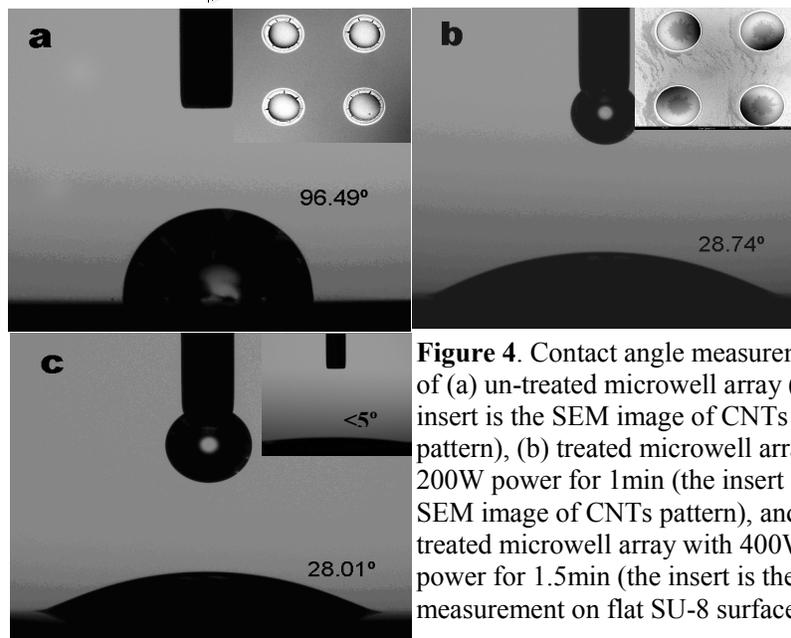
**Figure 4.** Contact angle measurements of (a) un-treated microwell array (the insert is the SEM image of CNTs pattern), (b) treated microwell array with 200W power for 1min (the insert is the SEM image of CNTs pattern), and (c) treated microwell array with 400W power for 1.5min (the insert is the measurement on flat SU-8 surface).
