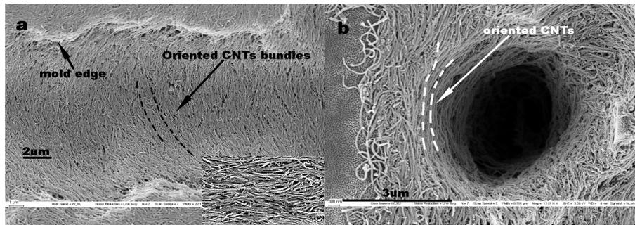
**Figure 2.** SEM images of aligned CNTs in (a) micro-channel and (b) circular well opening.
