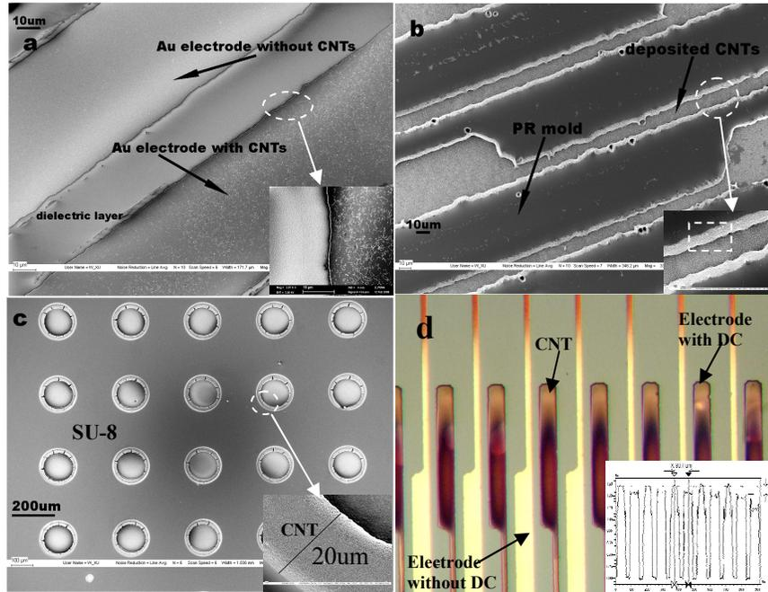
**Figure 1.** SEM images of CNTs assembly in (a) interdigital microelectrodes, (b) photoresist (PR) microchannels, (c) SU-8 microwell arrays and (d) optical image of the CNTs patterns in microelectrodes, the insert shows an electrode thickness measurement, illustrating the height difference between deposited and non-deposited electrodes.
