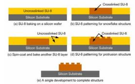
Figure 1. Process flow for a two-step SU-8 process
