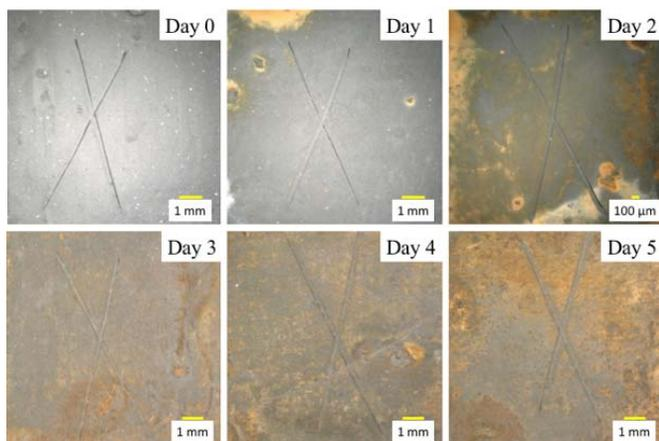
Fig. 3. Optical images of physiologically conditioned Fe-PCL composites (40%vf of Fe) after adhesion tests were performed on PLA substrates with micropatterned Fe traces.
