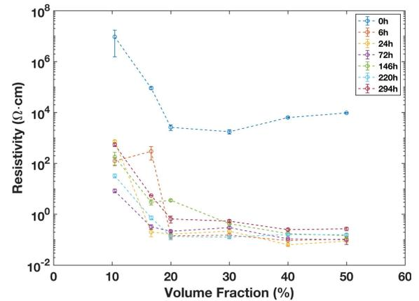
Fig. 2. Electrical resistivity of Fe-PCL biodegradable conductive polymer composite films at varying volume fractions of Fe, parameterized by degradation time.
