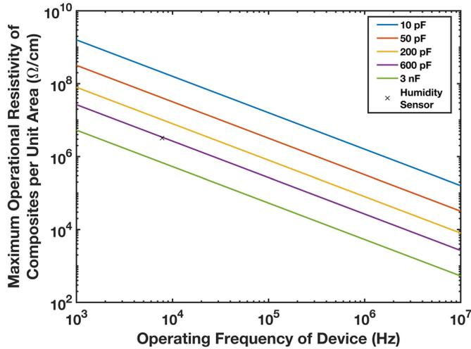
Fig. 9. Maximum operational resistivity of 0.1-mm-thick Fe-PCL biodegradable conductive polymer composites per unit area as a function of the operating frequency of the device, parameterized by input capacitance of the device.
