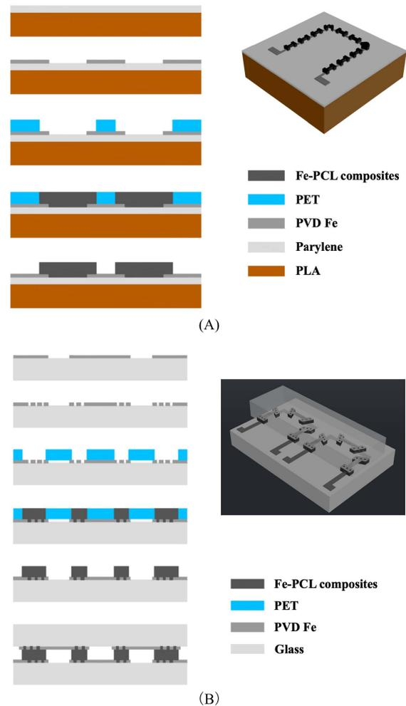
Fig. 1. Fabrication scheme and daisy-chain structures of Fe-PCL biodegradable electrical interconnects. (a) In-plane structure. (b) Out-of-plane structure.
