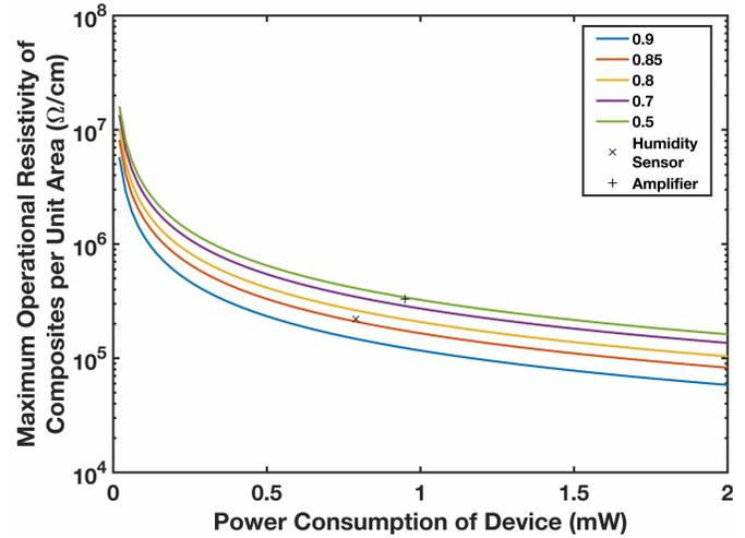
Fig. 8. Maximum operational resistivity of 0.1-mm-thick Fe-PCL biodegradable conductive polymer composites per unit area as a function of power consumption of the device, parameterized by the ratio of the device's voltage and supply voltage.
