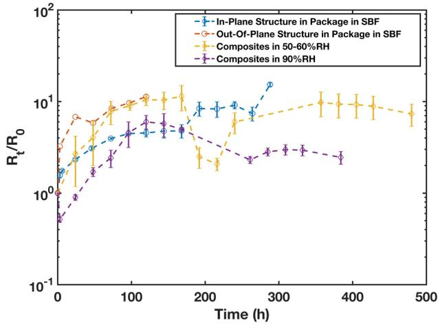
Fig. 7. Ratio of resistance change of packaged in-plane daisy-chain structure in SBF and Fe-PCL composite films degraded in humid conditions as a function of degradation time.
