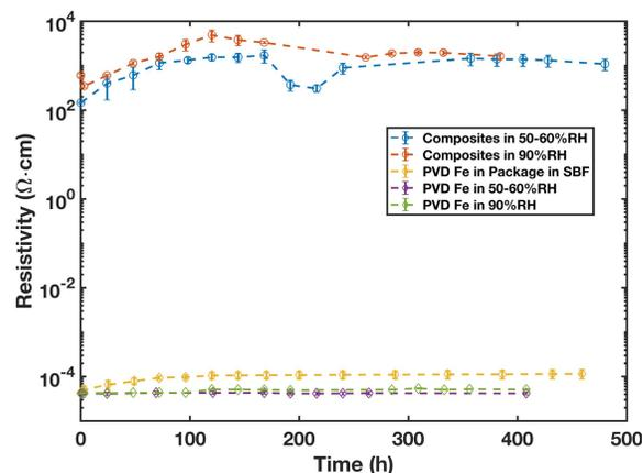
Fig. 4. Electrical resistivity of Fe-PCL biodegradable conductive polymer composite films (40%vf of Fe) and sputter-deposited Fe traces as a function of degradation time under various conditions.
