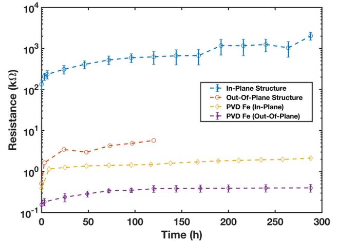
Fig. 6. Electrical resistance of packaged biodegradable daisy-chain structures and packaged sputter-deposited Fe traces as a function of degradation time.
