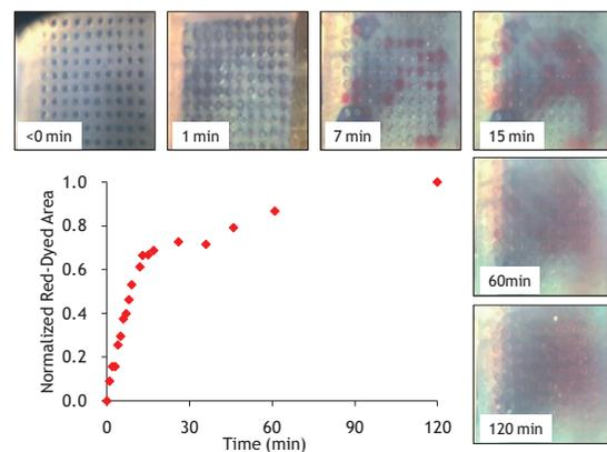
**Figure 6.** Diffusion kinetics of drug release into the agarose gel by the dissolvable-tipped microneedle array using diffusion of red-dyed surrogate.
