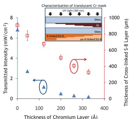
**Figure 2.** Characteristics of a gray-tone mask process. Measured transmitted intensity of UV light through a translucent chromium layer (▲) and thickness of a crosslinked SU-8 layer (◻) are plotted using the exposure scheme shown in the inset schematic.
