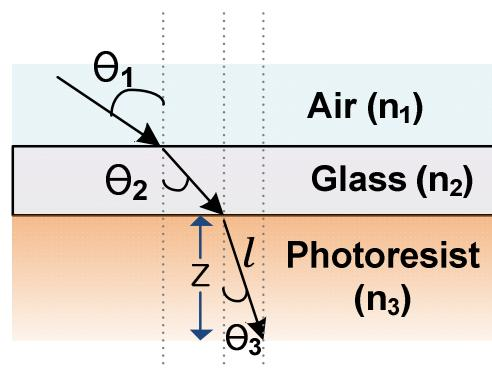
Figure 4. Inclined light propagation in the multidirectional UV lithography
