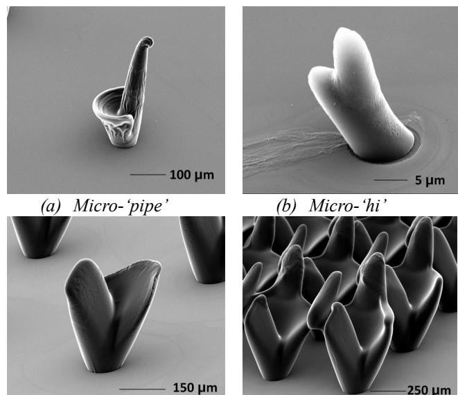
Figure 6. Complex 3-D microstructures using CNC lithography
