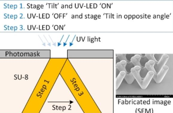
Figure 4. An example of CNC lithography program description for micro-'V' pillars: fabrication steps (left) and an SEM view of fabricated structures (right)
