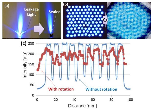
Figure 3. Light intensity distribution: (a) UV-LED sidewall coating and light propagation comparison, (b) optical image of intensity comparison without and with rotation, (c) intensity comparison plot
