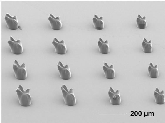
Figure 7. Batch fabrication of micro-cat's-claw
