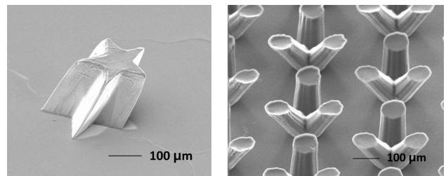
Figure 5. Fabrication result: inclined structures
