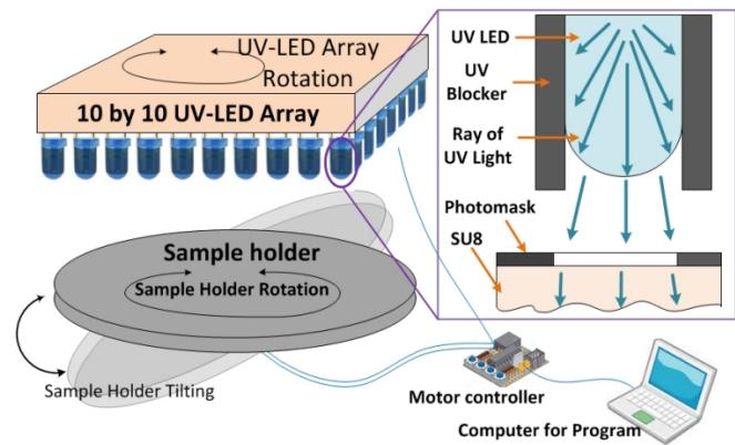
Figure 1. Schematic diagram of CNC-Lithography
