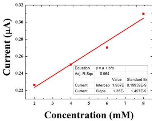
Fig. 4. Current response according to free-cholesterol concentration in 0.1M PBS (pH 7.4) at applied potential of 0.4V and correlation coefficient of current response
