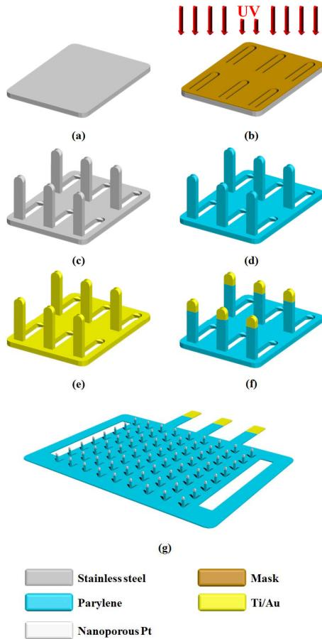
Fig. 1. Fabrication sequences of proposed non-enzymatic free-cholesterol sensor on micro-needle patch: (a) cleaning substrate, (b) photolithography for patterning of SUS, (c) forming micro-needles, (d) parylene/Ti/Au deposition,
