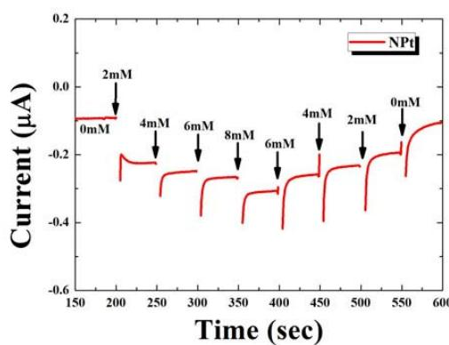
Fig. 5. Recovery characteristic of fabricated micro-needle patch sensor with stepwise change in each free-cholesterol concentration of 0, 2, 4, 6, and 8mM.
