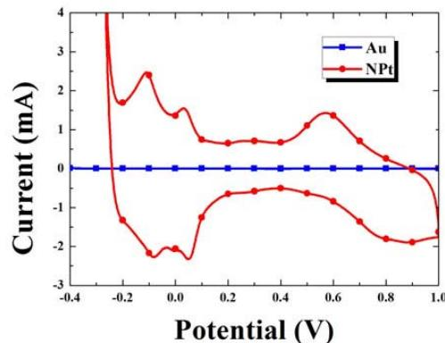
Fig. 3. Comparison of cyclic voltammetry of bare gold and Npt formed on micro-needle patch in 1M sulfuric acid at scan rate of 200mV/s in potential range of -0.4V to 1.0V.
