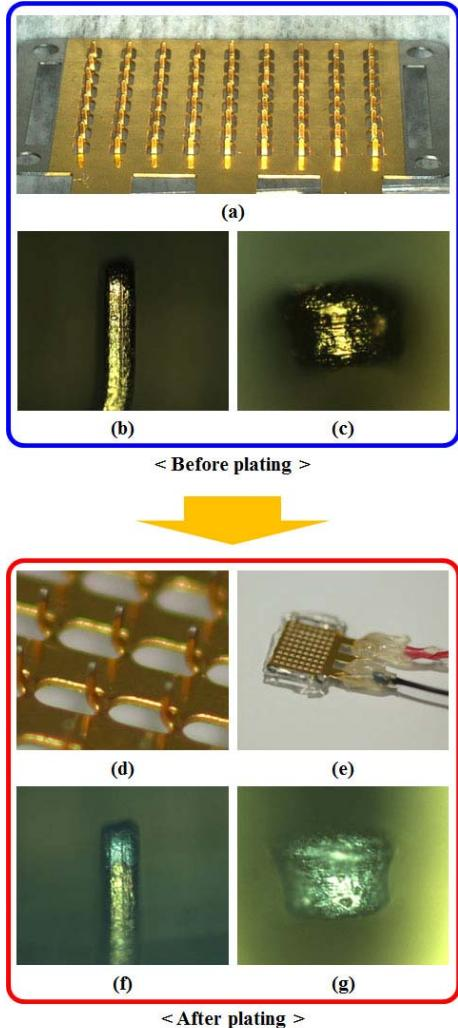
Fig. 2. Optical microscopic images before and after electroplating of micro-needle: (a) whole image before electroplating, (b, c) side and top view of a micro-needle before elecroplating, (d, e) whol image of after electroplating, (f, g) side and top view of a micro-needle after electroplating
