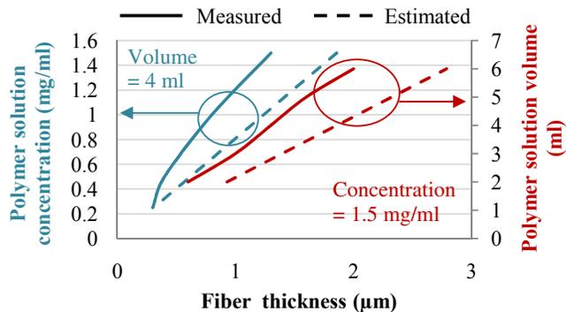
**Figure 3.** Variation of fiber wall thickness with collagen solution concentration for a fixed volume of 4 ml, and volume of the collagen solution for a concentration of 1.5 mg/ml.
