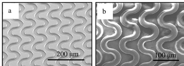
**Figure 5.** SEM images of, a) a serpentine silicon template, and b) in-plane serpentine collagen fibers with a designed strain of 57%.
