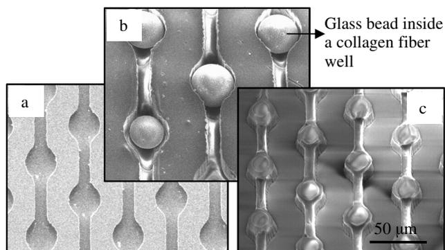
**Figure 7.** SEM images of, a) a silicon template for the fabrication of fibers for particle encapsulation, b) glass beads placed in periodic wells along hollow collagen fibers inside the trenches of the template, and c) glass bead encapsulated collagen fibers extricated using tape.
