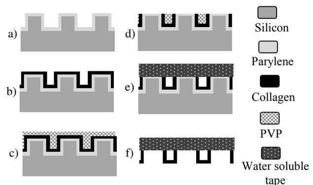
**Figure 1.** Fabrication process sequence, a) Deposit parylene on the silicon template, b) Solvent cast collagen solution, c) Spray coat PVP protectant, d) Individualize fibers by dry mechanical grinding or RIE, e) and f) Extract fibers using a water soluble tape after dissolving away PVP.
