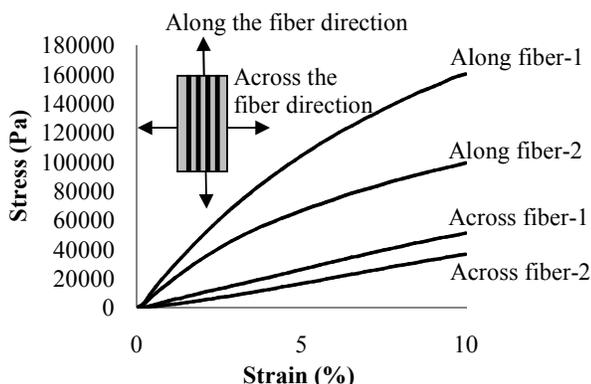
**Figure 10.** Stress-strain relationship of collagen-elastin composite illustrating material stiffening along the fiber direction as compared to across the fiber direction.
