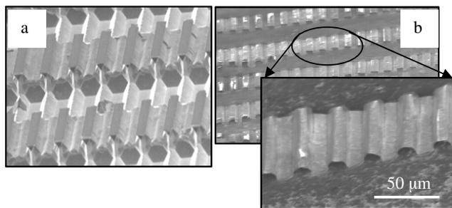
**Figure 6.** SEM images of, a) a multi-depth silicon template for the fabrication of out-of-plane wavy fibers, and b) out-of-plane wavy collagen fibers.
