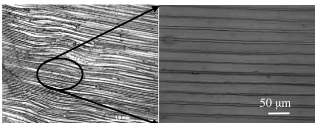
**Figure 9.** Microscope image of an aligned collagen microfiber composite in elastin matrix.
