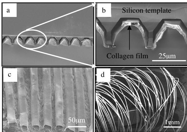
**Figure 2.** SEM images of, a) and b) cross section view of solvent cast collagen film on a silicon template with tip sharpened trenches, c) 25 μm wide individualized hollow collagen fibers extracted from the template using tape, alignment of the fibers is retained, d) 25 μm wide collagen fibers separated from the template by direct peeling.
