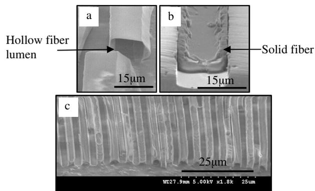
**Figure 4.** SEM images of, a) a hollow collagen fiber, b) a ribbon like solid collagen fiber, and c) 2 μm hollow fibers on tape.
