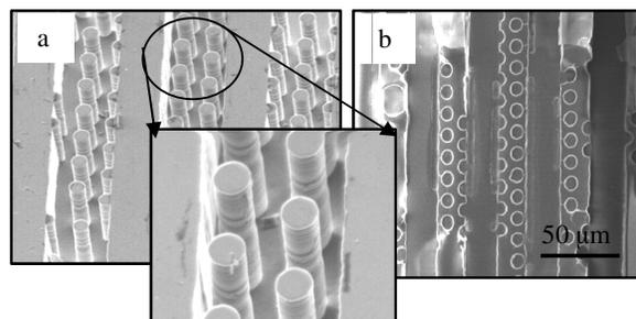
**Figure 8.** SEM images of, a) a silicon template with pillars in the trenches, and b) porous collagen fibers on tape.
