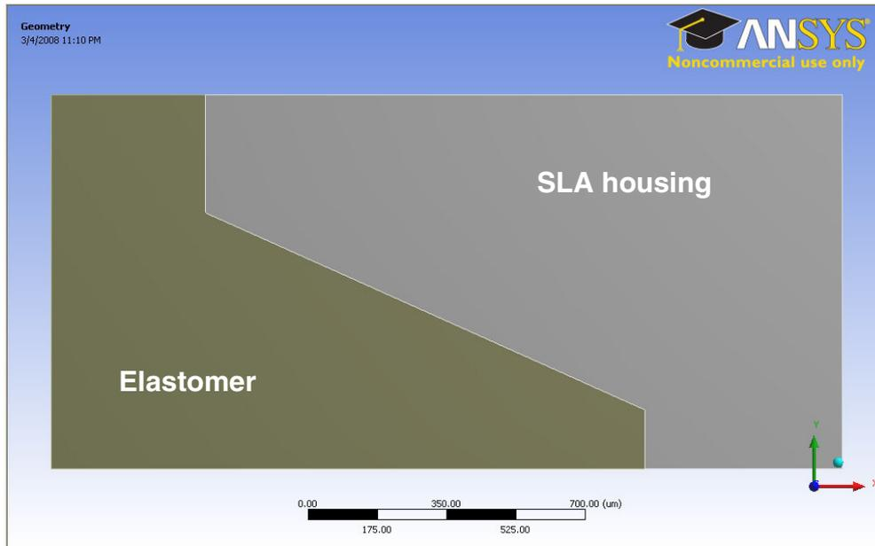
Figure 2. 2D geometry model of a SHA chamber filled with PDMS.
