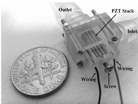
Figure 4: Photograph of a three-layer piezoelectrically driven hydraulically amplified polymer microvalve. Dimensions of the valve are 6mm×13mm×9mm.
