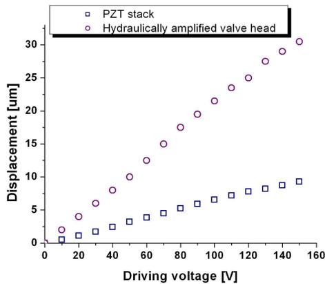
Figure 5: Displacement measurements of PZT driving element and hydraulically amplified valve head.
