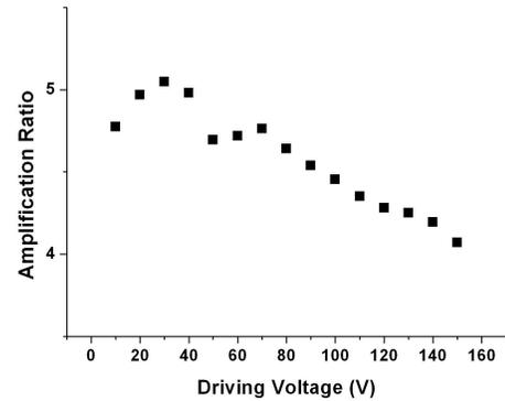
Figure 6: Calculated amplification ratio as a function of driving voltage.
