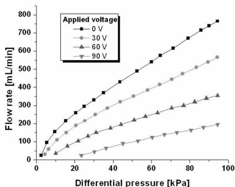
Figure 8: Measured  $N_2$  flow rate as a function of differential pressures at different actuation voltages (dc).
