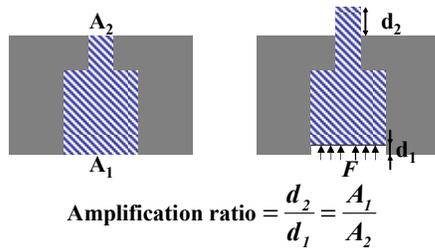
Figure 1: Principle of the solid hydraulic amplification mechanism.
