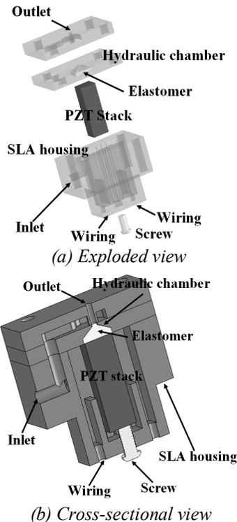
Figure 2: 3-D schematics of the microvalve configuration, showing the geometry of the hydraulic chamber and the inlet and outlet paths.
