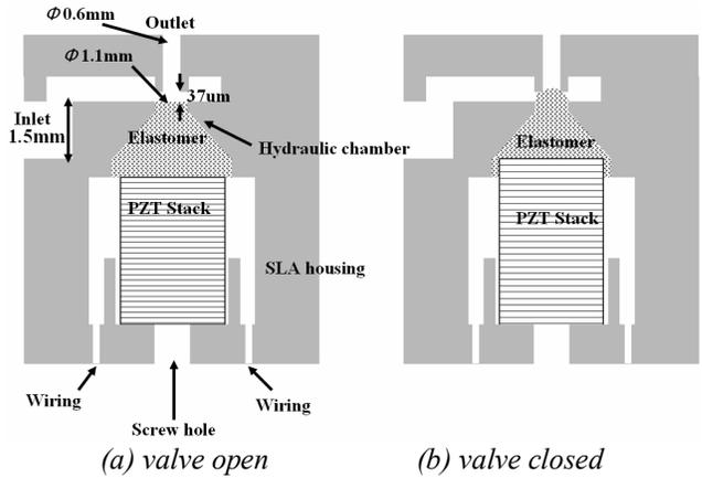
Figure 3: Operating principle of the normally open piezoelectric polymer microvalve.
