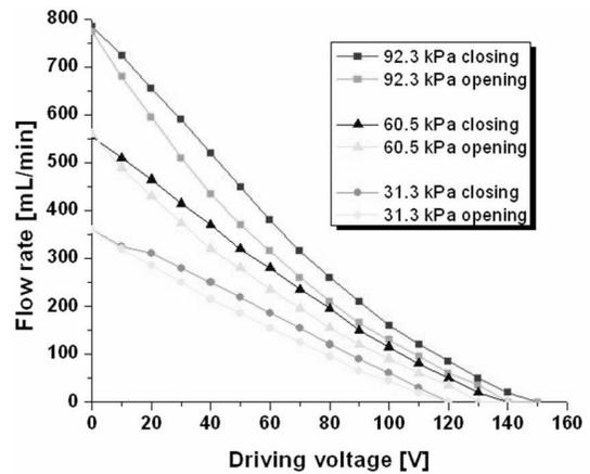
Figure 7: Measured N<sub>2</sub> flow rate as a function of actuation voltage (dc) under various differential pressures.
