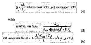
A high performance substrate, suspended topology and proper spacing between turns greatly reduce parasitic capacitances. This leads to enhanced quality factor and very high frequency of operation.
