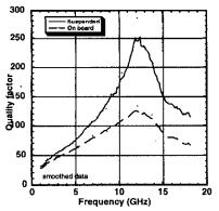
Fig.10. Measured performances for 1 turn suspended inductor compared with one turn on-board inductor.
