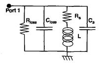
Fig.7. Equivalent hybrid model for 1 port suspended spiral inductor.
