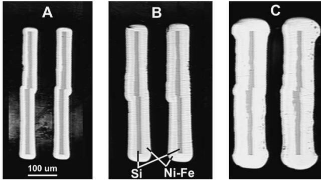
Fig. 2. Optical images showing partial cross-sections of laminated Ni-Fe structures with different  $w_{lam}$  (A = 23  $\mu\text{m}$ , B = 38  $\mu\text{m}$ , and C = 53  $\mu\text{m}$ ). Some misalignment is noted between the top- and bottom-side etch.
