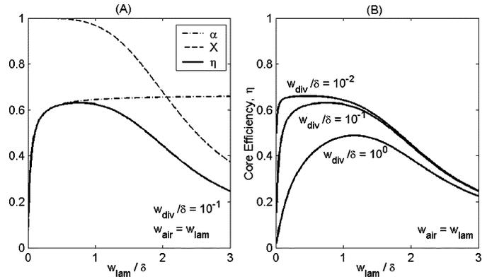
Fig. 3. Core efficiency is limited by packing density and eddy current losses. (a) Overlay of packing density  $\alpha$ , magnetic flux efficiency  $X$ , and total core efficiency  $\eta$ , showing poor packing density at low  $w_{lam}/\delta$  and large eddy current losses at large  $w_{lam}/\delta$ . (b) Core efficiencies  $\eta$  for various silicon divider widths.
