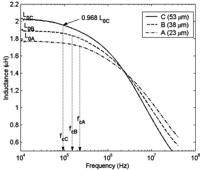
Fig. 4. Inductance versus frequency for three samples of increasing lamination thickness (and increasing packing density). The key parameters for each curve are the low-frequency (DC) inductance  $L_0$  and cutoff frequency  $f_c$  (at frequency  $f_c$ ,  $L(f_c) = 0.968 L_0$ ).
