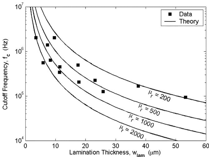
Fig. 5. Measured cutoff frequencies  $f_c$  decrease with lamination thickness  $w_{\text{lam}}$ . Theoretical cutoff frequencies (assuming constant relative permeabilities of 200, 500, 1000, and 2000) are shown for reference.
