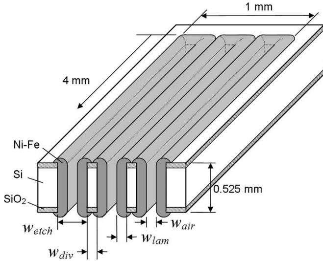
Fig. 1. Schematic of vertically laminated Ni-Fe core. For illustration,  $w_{etch} = 3w_{div} = 3w_{lam} = 3w_{air}$ , depicting a packing density of 50%.
