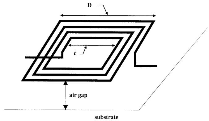
Fig. 1. Schematic drawing of the fabricated spiral-type air core inductor with a large air gap between the conductor lines and the substrate.
