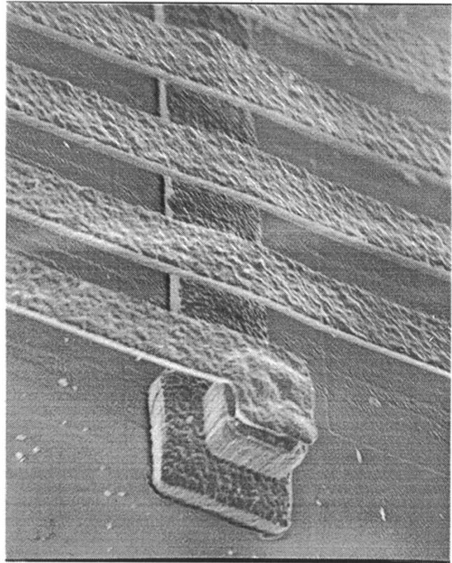
Fig. 6. Scanning electron micrograph of large suspended plated spiral conductor lines and signal connection through plated via (all metals are plated copper).
