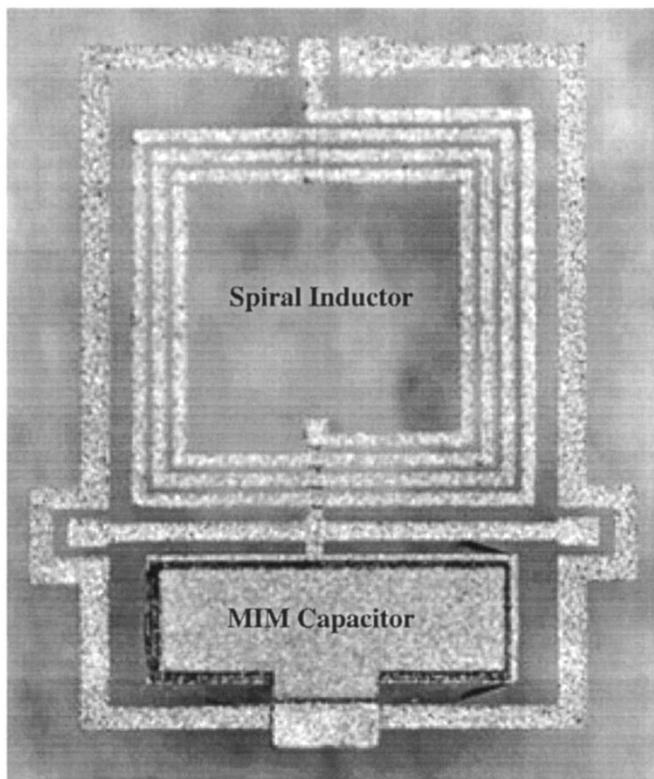
Fig. 7. Photomicrograph of fully integrated RF-LC filter using composite MIM capacitor and spiral-type air core inductor suspended over the substrate (dimension: 1.9 mm  $\times$  2.4 mm).
