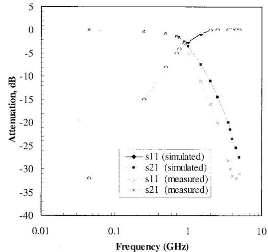
Fig. 11. Characteristics of the fabricated LC microfilter: 3 dB attenuation at 880 MHz.
