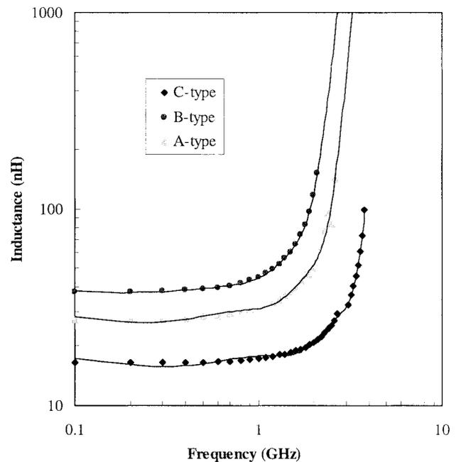
Fig. 8. Comparison of inductance of the fabricated spiral-type air core inductors suspended from the substrate.
