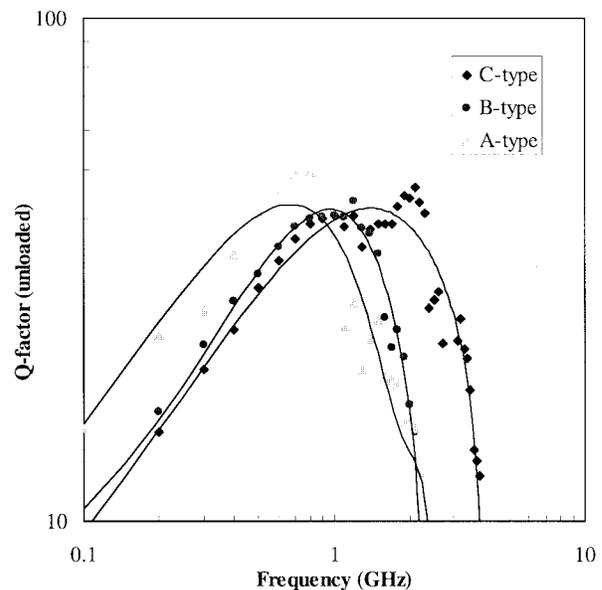
Fig. 9. Comparison of quality factor of the fabricated spiral-type air core inductors suspended from the substrate.
