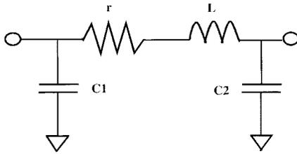
Fig. 10. Lumped element equivalent circuits for the fabricated large suspended spiral-type air core inductor.
