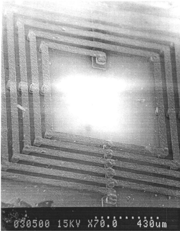
Fig. 4. Scanning electron micrograph of the fabricated large suspended spiral-type air core inductor.
