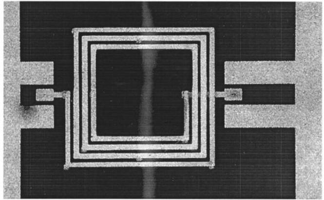
Fig. 3. Photomicrograph of the fabricated large suspended spiral-type air core inductor.
