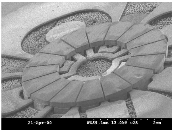
Figure 2. A micrograph of a first-generation non-laminated stator. The coil insulation has been partially etched back to reveal the coils
