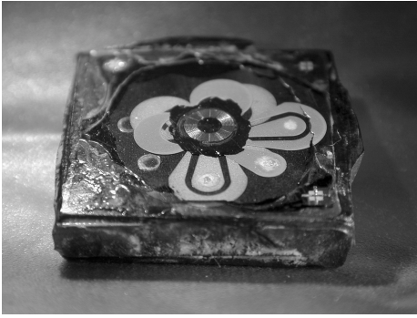
Figure 7: Optical photograph of a complete stator with laminated NiFe core. The device is built on top of a 5 mm thick ferrite wafer.
