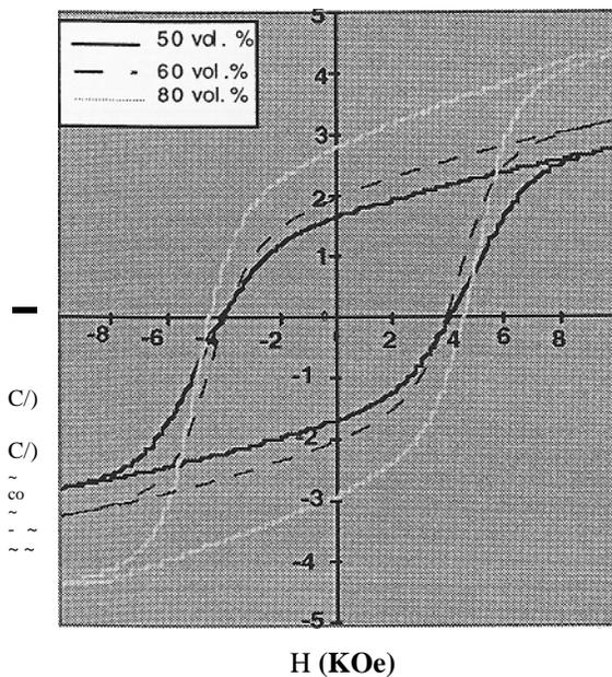
Figure 1. Magnetization curves for different ferrite loading concentrations.
