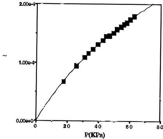
Figure 2. Typical load/deflection characteristics for the magnetic polymer composite (55 vol. 0/0 loading)
