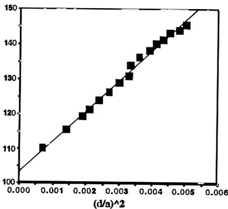
Figure 3. Load/deflection data plotted in accordance with Eq.(1) for the magnetic polymer composite (55 vol. % loading)
