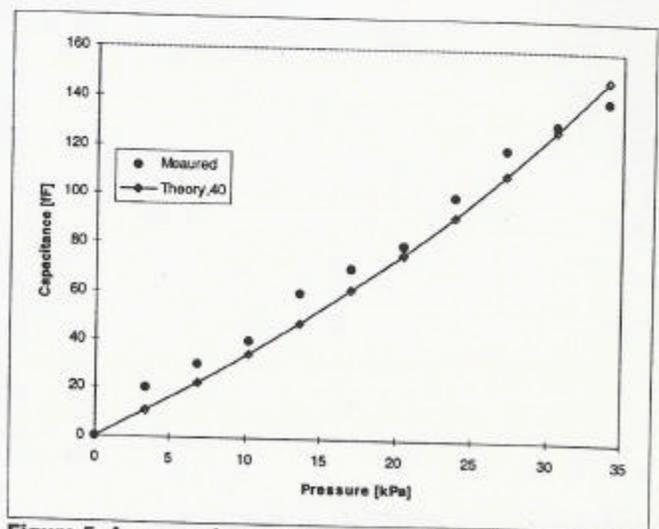
Figure 5. A comparison of theoretical and measured values of net capacitance change over the full range of applied pressure ranging from 0 to 34 kPa.
