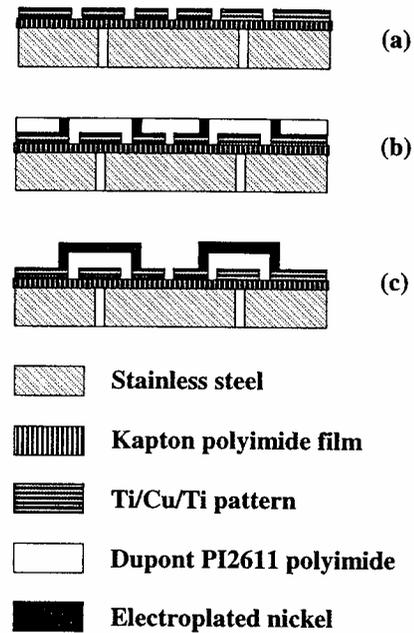
**Figure 2. Fabrication sequence: (a) lamination of milled stainless steel and Kapton polyimide film and bottom electrode patterning; (b) polyimide deposition and electroplating of nickel posts; (c) backplate electroplating and removal of polyimide sacrificial layer.**
