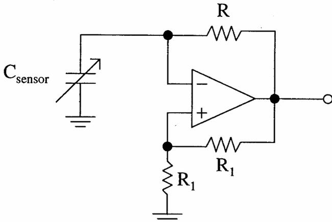
Figure 6. Schematic diagram of the astable multivibrator circuit.
