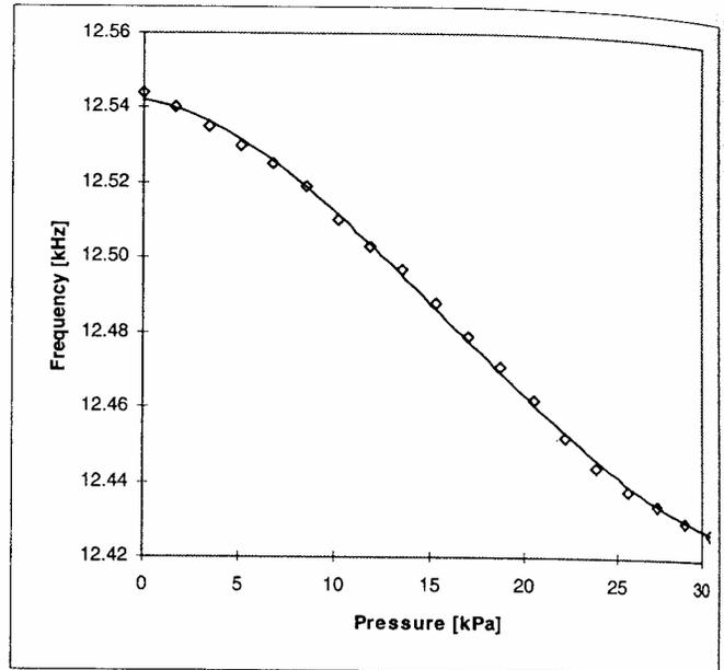
Figure 7. Frequency output of the hybrid multivibrator circuit in response to pressure sensor capacitance change over the applied pressure ranging from 0 to 30 kPa.
