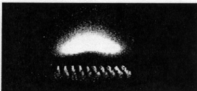
Figure 8 - A photomicrograph of an array of microneedles combusting a mixture of propane and air.
