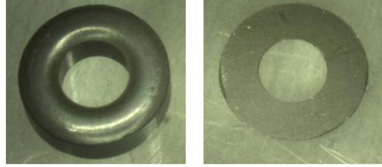
Figure 2. An iron powder core from Micrometals®: before (left) and after (right) lapping. The core thickness is 1.78mm before lapping and 200 -250  $\mu\text{m}$  after lapping. The inner diameter of these cores is 2.24 mm, and the outer diameter is 5.08mm.
