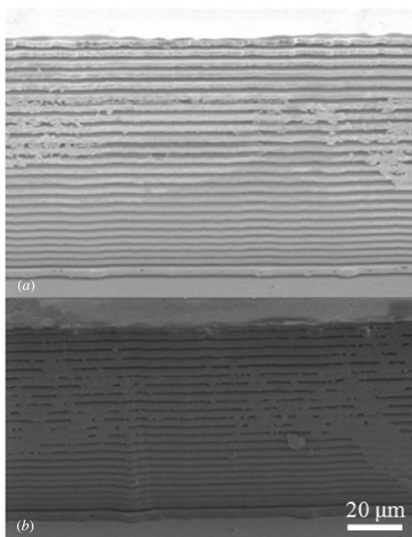
**Figure 5.** SEM images of the sidewall of the multilayer structure: (a) before and (b) after active material deposition.
