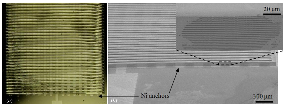
**Figure 2.** Optical and SEM images of the multilayer Ni backbone: (a) optical image illustrating the top view of the electrode where the vertical and horizontal lines represent the anchors and multilayer backbones, respectively, (ii) SEM image demonstrating the multilayer Ni backbone after complete removal of the selective Cu layers.
