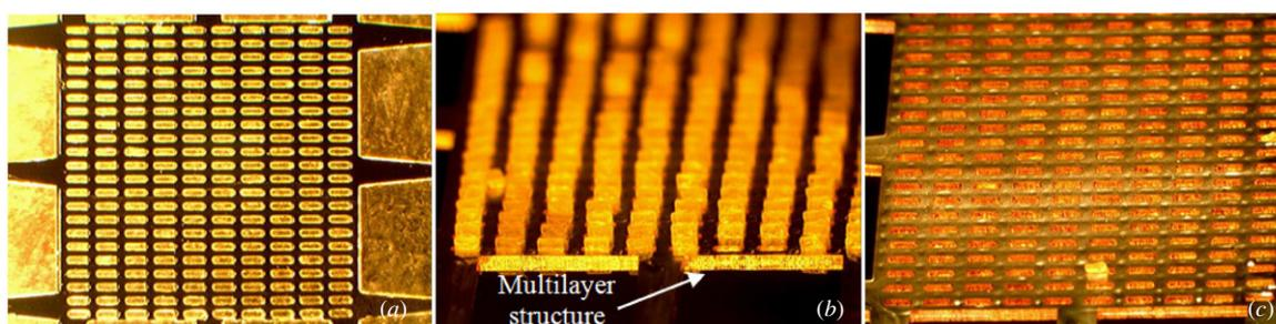
**Figure 4.** Optical images showing the ultra-thick mold: (a) top view of the array of high aspect ratio pillars before electroplating, (b) electroplated multilayer structure before the removal of the mold, (c) multilayer structure with etching holes exposed after the stripping of the mold.
