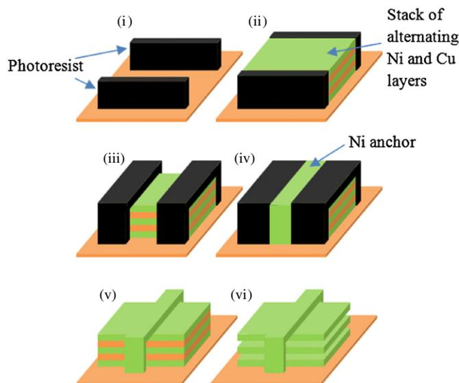
**Figure 1.** Fabrication schematic of the current collector demonstrating six major steps: (i) photoresist mold deposition and patterning, (ii) electroplating of alternating Ni and Cu layers, (iii) second photoresist mold patterning, (iv) electroplating of Ni anchor, (v) removal of photoresist, (vi) selective and complete etching of sacrificial Cu layers.
