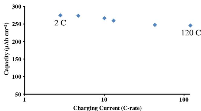
**Figure 7.** Areal capacity of the 25-layer electrode at various charge rates.
