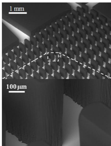
**Figure 3.** SEM images of the high aspect ratio mold before the electroplating process.
