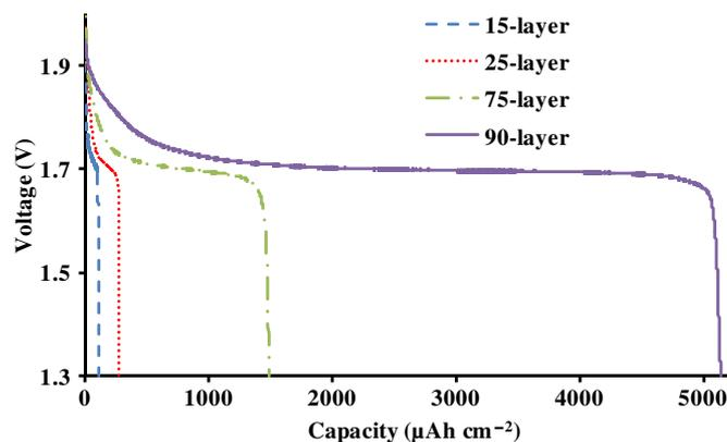
**Figure 6.** Performance of the electrodes with varying number of layers.
