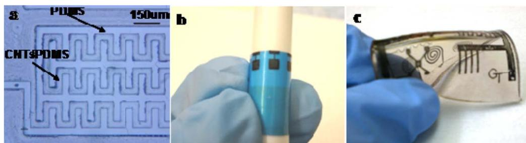
**FIGURE 2** (a) The optical image of CNT microspring patterns on PDMS, (b) the digital image of CNT patterns on a polyolefin film, and (c) the digital image of CNT patterns on a PDMS substrate. [Color figure can be viewed in the online issue, which is available at [wileyonlinelibrary.com](http://wileyonlinelibrary.com).]
