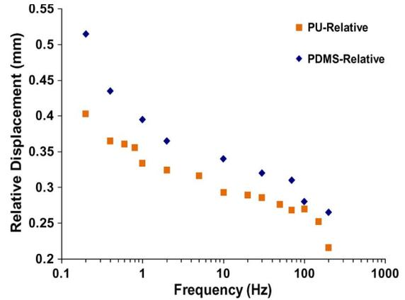
Fig. 13. Frequency response of Braille dots.
