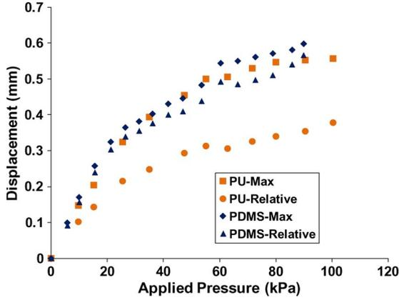
Fig. 14. Relative displacements of a PU Braille dot and a PDMS Braille dot at 0.2 Hz.
