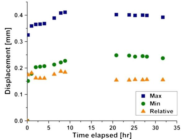
Fig. 16. Long-term actuation stability of the Braille dot.
