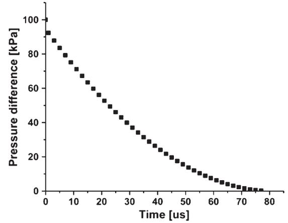
Fig. 15. Pressure difference between gas supply pressure and actuator pressure as a function of time after the valve is open.
