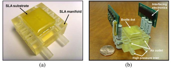
Fig. 6. Assembly of the actuator layer to manifold and microvalves. (a) Bonded actuator layer and manifold. (b) Final assembled device with microvalves.
