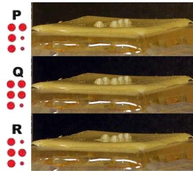
Fig. 7. Actuation of Braille dots corresponding to Braille alphabets.
