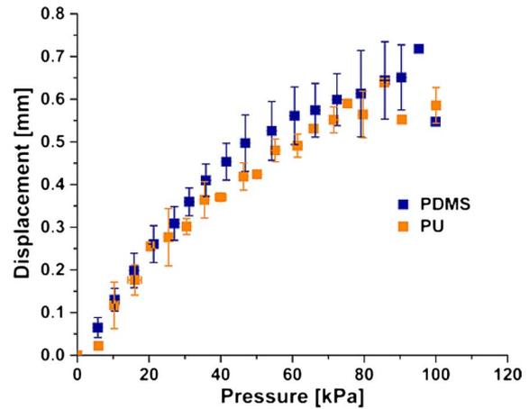
Fig. 10. Averaged dot heights for a PDMS Braille cell and a PU Braille cell as a function of applied pressure.
