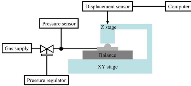
Fig. 11. Diagram of force measurement.
