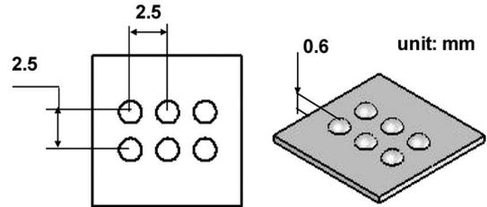
Fig. 1. International building standard for a Braille cell.
