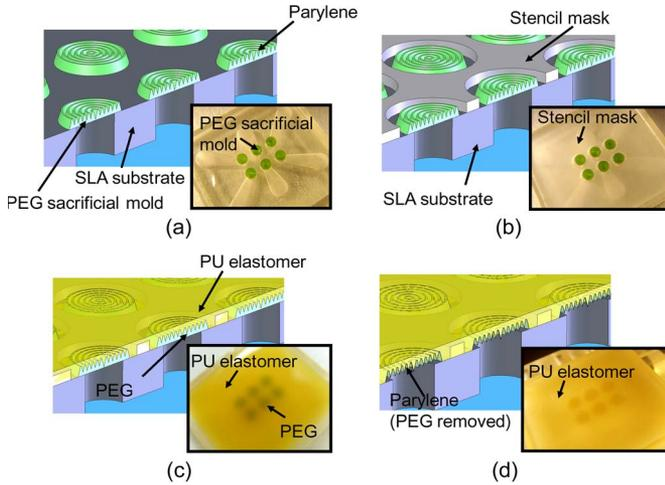
Fig. 5. Fabrication process steps. (a) PEG micro transfer molding and parylene coating. (b) Planarization with SLA stencil mask. (c) PU coating and curing. (d) Removal of PEG sacrificial mold.
