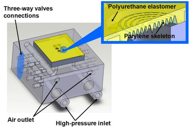
Fig. 3. Schematic of the laminated pneumatic actuator layer on the fluidic manifold.
