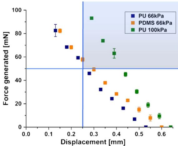
Fig. 12. Force generated by an actuated PU Braille dot and an actuated PDMS Braille dot.
