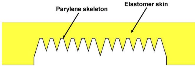
Fig. 2. Cross-sectional schematic of an endoskeletal microbubble actuator.
