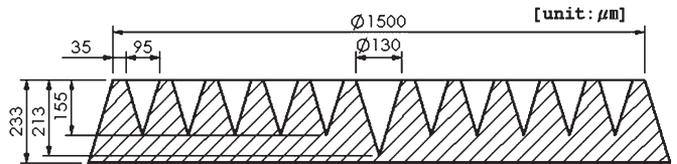
Fig. 4. Profile and dimensions of the designed corrugated diaphragm [6].
