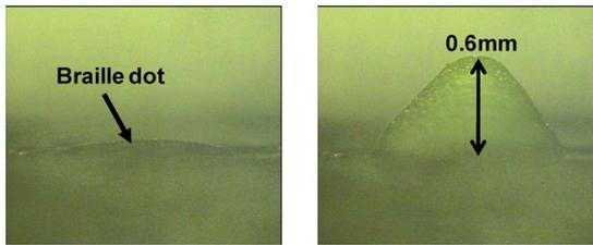
Fig. 8. Microscopic images of the inactivated and the actuated Braille dot. (a) Inactivated Braille dot. (b) Actuated dot at 100 kPa.
