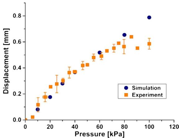
Fig. 9. FEM and experimental results of averaged dot heights for a PU Braille cell.
