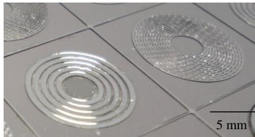
Figure 4: 100-layer magnetic permalloy core electroplated using robotically-assisted multilayer electroplating setup and controlled-roughness electrodeposition. The total device thickness is on the order of 100 microns
