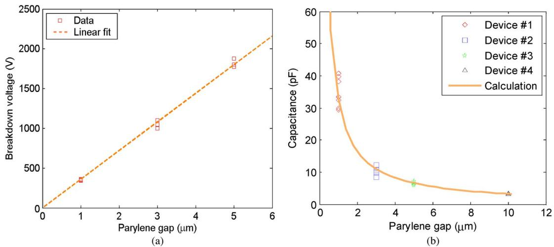
Fig. 6. (a) Voltage breakdown and (b) capacitance measurements between the first and second electroplated layers of the comblike structures as a function of the parylene thickness.
