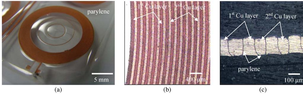
Fig. 8. Images of the ultradense parylene-encapsulated spiral coils. (a) Front side. (b) Close-up view. (c) Cross-sectional view.
