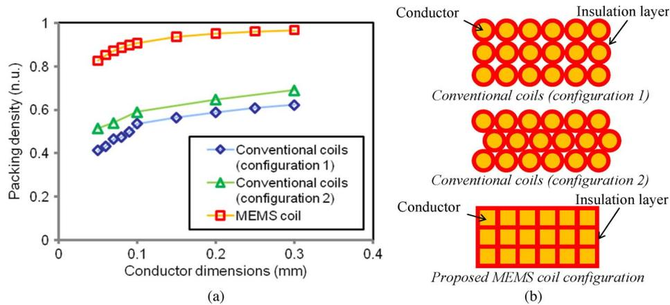
Fig. 1. (a) Packing density as a function of the conductor dimensions calculated over an array of conductors and (b) schematics of the three configurations. The round magnet wires have standard insulation [1], while the MEMS-fabricated square coils have a 5- $\mu\text{m}$ -thick parylene insulation.
