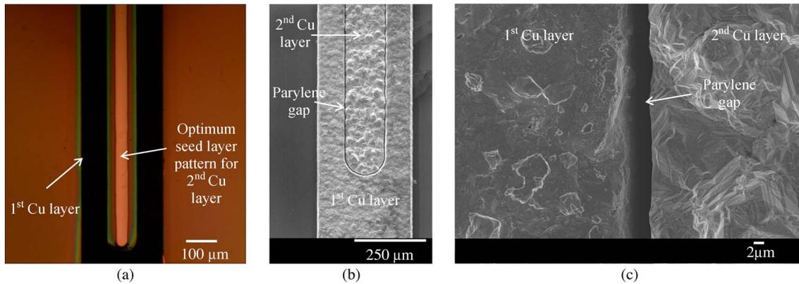
Fig. 5. Ultradense comblike electroplated test structures. (a) Before and (b) and (c) after plating. (b) and (c) Parylene was removed by plasma etching after the second copper electroplating for imaging purposes.
