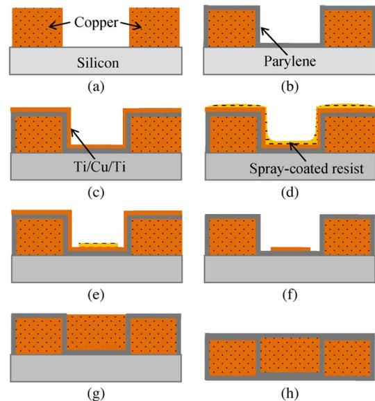
Fig. 2. Fabrication process flow of ultradense microcoils. (a) Standard through-resist mold electroplating. (b) Parylene insulation. (c) Ti/Cu/Ti deposition. (d) Spray coating of negative-tone photoresist. (e) Photoresist patterning. (f) Seed layer patterning. (g) Second electroplating sequence. (h) Release and insulation of the fabricated coils.
