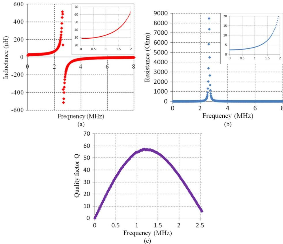
Fig. 9. Impedance characterization of ultradense parylene-encapsulated microcoils. (a) Inductance. (b) Resistance. (c) Quality factor as a function of frequency.
