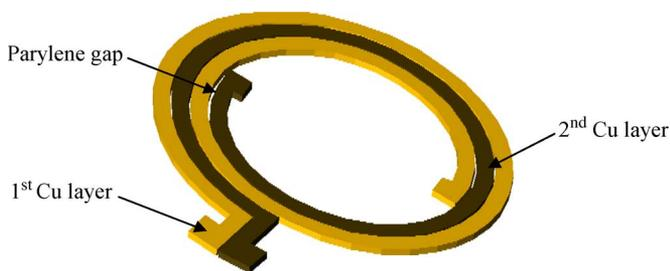
Fig. 7. Rendering of the microfabricated ultradense spiral coil.
