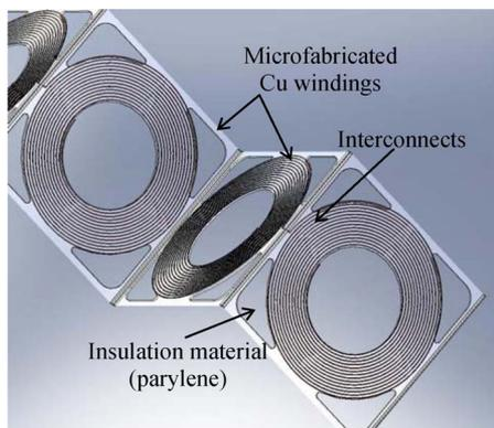
Fig. 3. Rendering of the folding concept to create 3-D MEMS-based coils from a flexible array of planar microfabricated windings.
