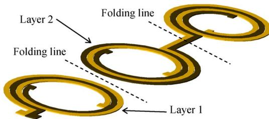
Fig. 10. Three-dimensional conceptual rendering of an ultradense three-layer spiral coil structure before folding.
