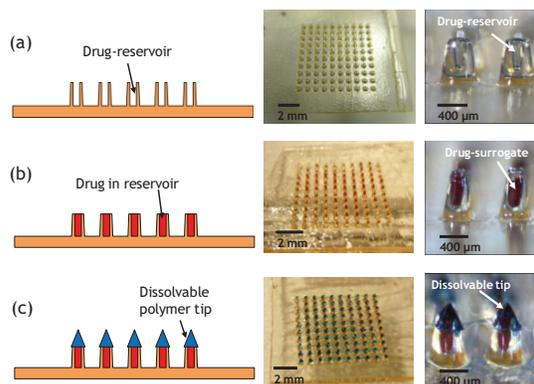
**Figure 4.** The fabricated microneedle array. (a) Before and (b) after filling reservoirs with a drug-surrogate. (c) Blue-dyed dissolvable tips are contact-transferred onto the drug-reservoirs.
