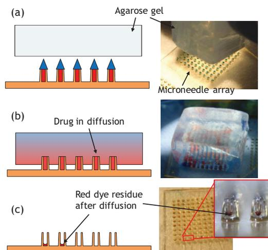
**Figure 5.** (a) A microneedle array to be inserted into agarose gel. (b) The water-soluble tips dissolve after insertion within a minute, and then drug-surrogate stored in reservoirs diffuse into gel. (c) The microneedle array following 2 hours of dye delivery into gel.
