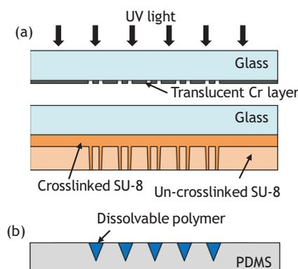
**Figure 3.** (a) Schematic of fabrication process for drug-reservoir integrated microneedles using a gray-tone mask. (b) Schematic of a reusable PDMS mold of trenches for sharp tips, which is filled with a dissolvable polymer.
