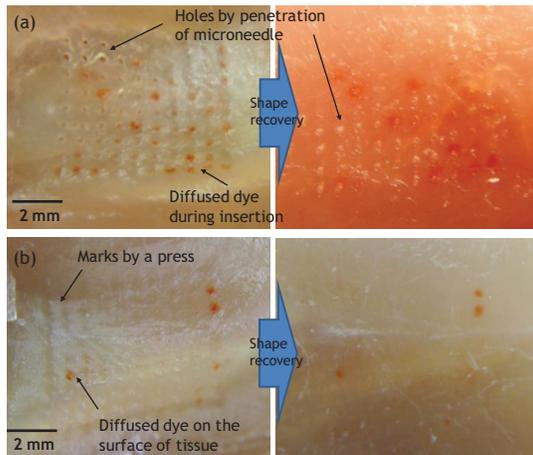
**Figure 7.** Insertion test of developed microneedle array into a chicken leg muscle. (a) Holes caused by penetration of microneedle tips maintain after shape recovery by tissue tension. (b) Insertion test with the used microneedle array. Pressed marks disappear after shape recovery.
