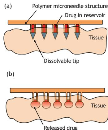
**Figure 1.** (a) Schematics of the microneedle array, consisting of reservoirs storing a drug, a substrate for mechanical support, and dissolvable tips. (b) Illustration of drug release after tips dissolving in a tissue.
