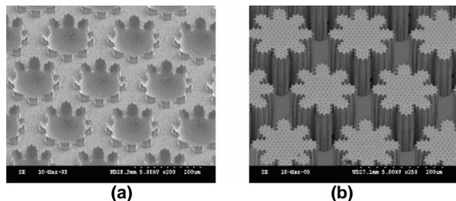
**Figure 6: (a) PU cast from Au coated PDMS mold with metal transfer and (b) from a PDMS mold without metal coating**
