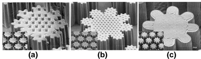
**Figure 5: PU structure from Au coated PDMS mold with metal transfer with 10, 5, and 2  $\mu\text{m}$  salient features on sidewall and protrusions on the top surface (from left)**
