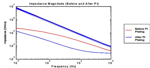
**Figure 9: Electrical impedance spectroscopy results of the 3-D MEA before and after platinum plating.**
