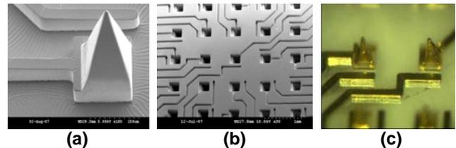
**Figure 8: (a) SEM image of a 3-D and 2-D electrode; (b) SEM image of the SU-8 mold; (c) Optical image of a PU 3-D MEA**
