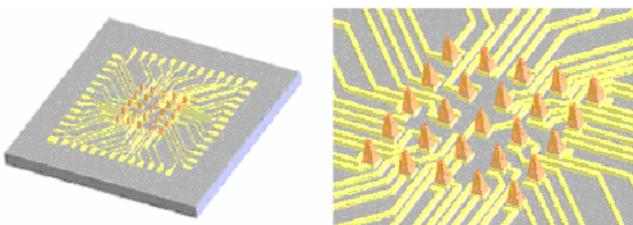
**Figure 7: Schematic of the proposed 3-D MEA**
