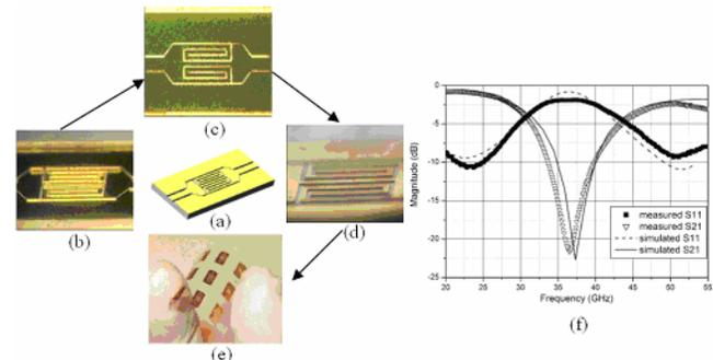
**Figure 12: MTM molded band stop filter array: (a) schematic design (b)-(e) fabrication flow of devices (f) measured and simulated S11 and S21**
