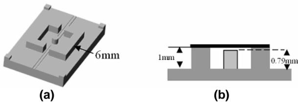
**Figure 13: Schematic of the CPW fed cavity resonator design (a) lateral view (b) side view**
