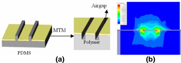
**Figure 11: (a) MTM process of coplanar waveguide (CPW) with air gap (b) simulated E-field in the air-gap CPW**
