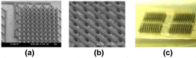
**Figure 2: An array of electrodes (100  $\mu\text{m}$  diameters) molded by photocurable epoxy resin. (a) Master structure by SU-8 (b) PDMS mold (c) molded epoxy resin structure with transferred gold on the surface**
