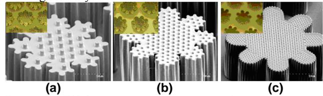
**Figure 3: SU-8 master structure on silicon substrate: 150  $\mu\text{m}$  tall columns with 10, 5, and 2  $\mu\text{m}$  salient features on sidewall and protrusions on the top surface (from left)**
