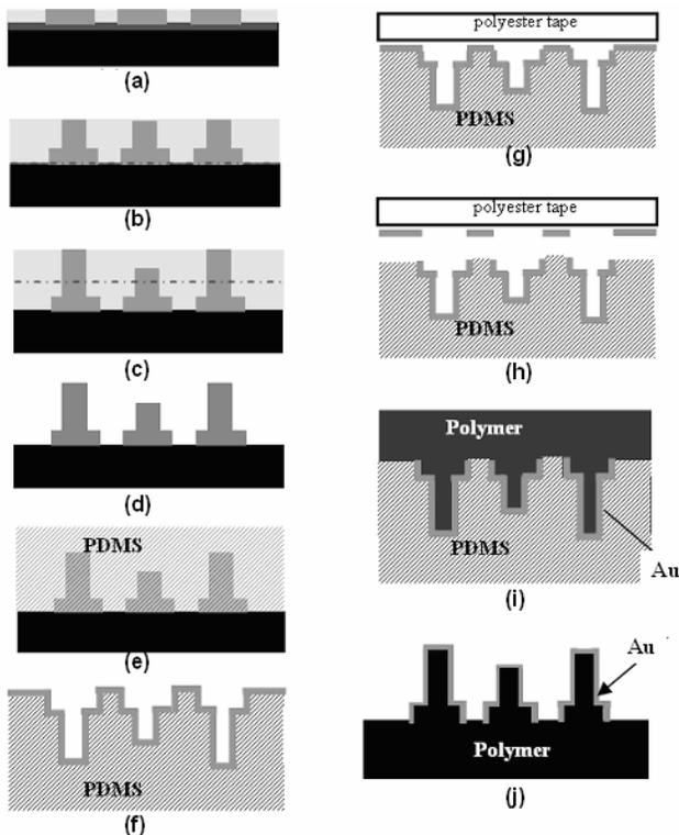
Figure 1: MTM process flow
