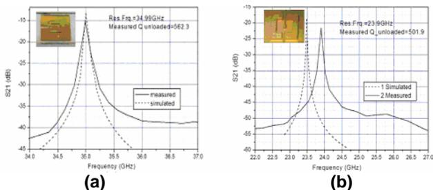
**Figure 14: Characteristics of MTM fabricated cavity resonators (a) conventional cavity resonator (b) evanescent-mode cavity resonator**
