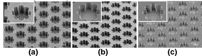
**Figure 4: Elastomeric PDMS mold coated with Au: column wells with 10, 5, and 2  $\mu\text{m}$  salient features on sidewall and dimples on the bottom (from left)**
