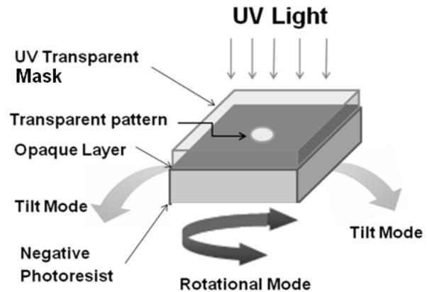
Figure 1: Dynamic mode multidirectional UV exposure
