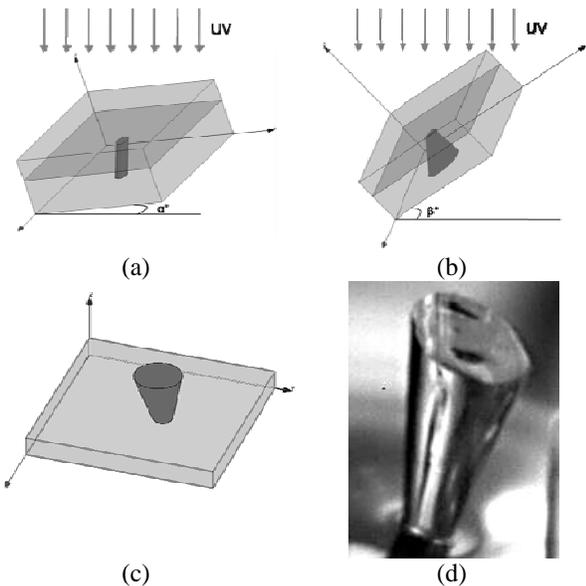
Figure 3: Fabrication process: (a) Expose the sample with a tilting angle of  $\alpha^\circ$ , (b) Change the tilting angle with continuous rotation during exposure, (c) Post exposure bake and develop to complete the process, (d) Fabricated asymmetric corn structure
