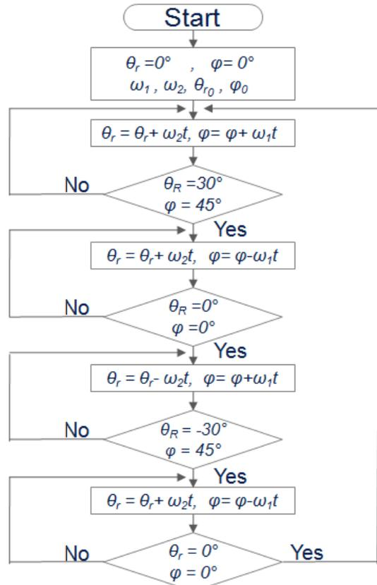
Figure 5: Automated dynamic mode operation algorithm for a screwed wind vane
