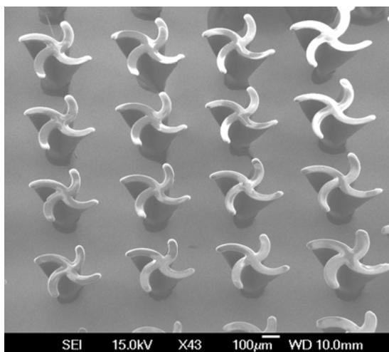
Figure 6: SEM Photograph of the 3-D microstructure array fabricated using automated dynamic mode multidirectional UV lithography
