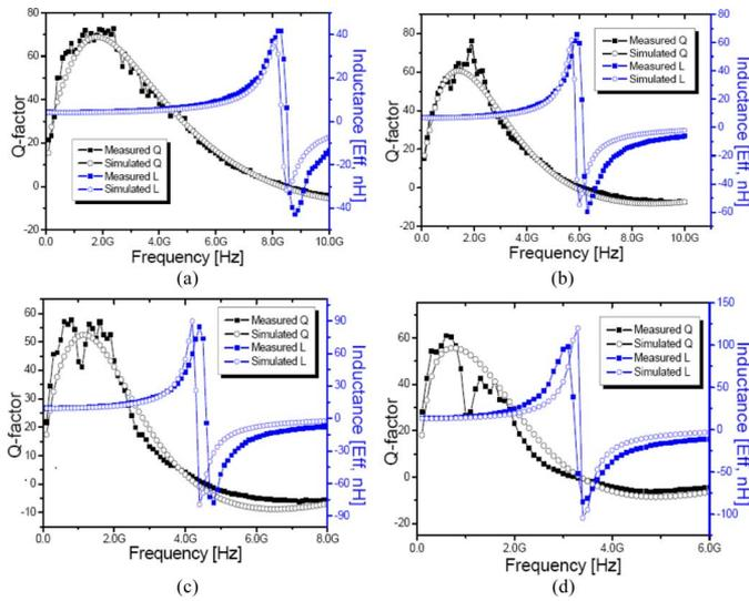
Fig. 8. Measured and simulated  $L_{\text{eff}}$  and  $Q$  of the inductors: (a) three-turn, (b) five-turn, (c) seven-turn, and (d) 10-turn inductors.
