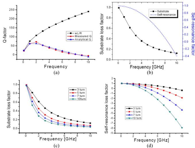
Fig. 9. Frequency response of inductors: (a)  $Q$ -factor and  $\omega L/R$  term of a three-turn inductor, (b) substrate loss factor and self-resonance loss factor of a three-turn inductor, (c) substrate loss factor of the inductors, and (d) self-resonance loss factor of the inductors.
