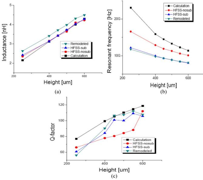
Fig. 3. HFSS results for remodeled structures.
