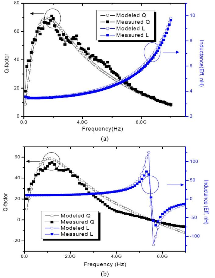
Fig. 6. Measured and modeled  $L_{\text{EFF}}$  and  $Q$  of (a) three-turn and (b) seven-turn inductors with solid metallic posts.
