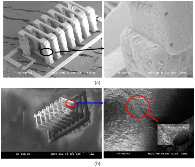
Fig. 5. SEM pictures of the interconnect layer inductors: (a) inductor with solid metallic posts and (b) inductor with polymer-core-conductor posts.
