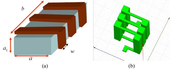
Fig. 1. Schematics of designed inductors for (a) Niwa's model (1) and (b) for HFSS.
