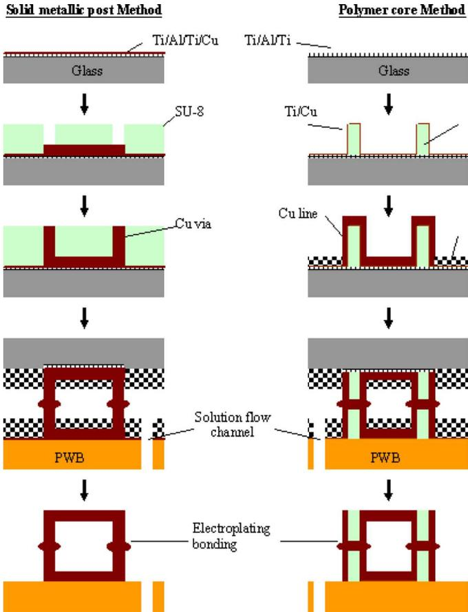
Fig. 4. Fabrication methods for interconnect layer inductors: (left) inductor with solid metallic posts, and (right) inductor with polymer-core-conductor posts.
