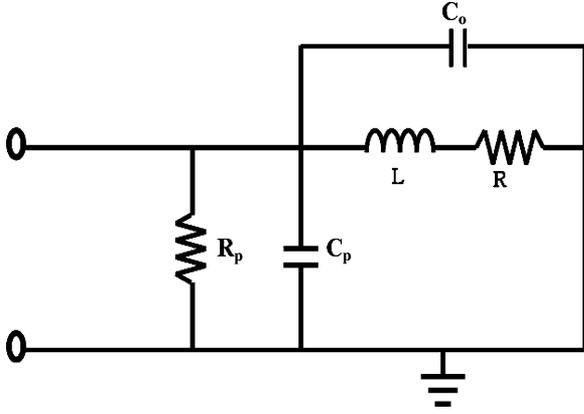
Fig. 7. Equivalent circuit model for an one-port inductor used for the performance evaluation.
