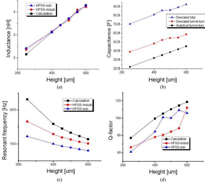
Fig. 2. Comparison of inductor characteristics of theoretical calculation, HFSS without a substrate, and HFSS with a substrate: (a) inductance, (b) capacitance, (c) resonant frequency, and (d)  $Q$ -factor.
