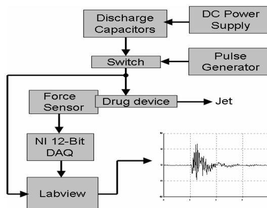
Fig. 5 Force sensing setup.
