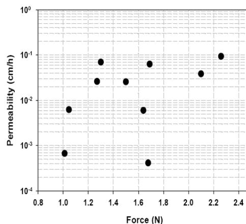
Fig. 6 Comparing skin permeability with force generated from the jet device.
