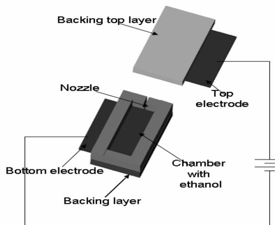
Fig. 1 Schematic of a single jet ejector system.
