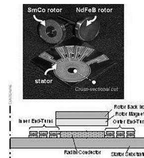
(a) Optimized winding geometry stator and rotors (b) Cross-sectional schematics.
