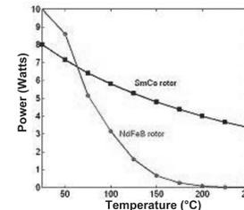
Output DC power as a function of temperature at 300 krpm
