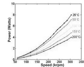
Output DC power delivered to external load as a function of speed parameterized by temperature for a SmCo rotor
