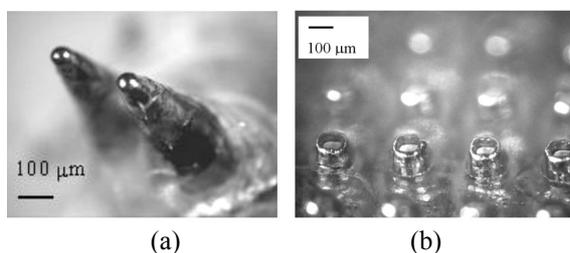
Figure 2. Photographs of microfabricated micro-heating elements: (a) Type A, two conical metal posts (tip diameter of  $80\mu\text{m}$ , base diameter of  $400\mu\text{m}$ , metal shell thickness of  $50\mu\text{m}$ , and height of  $2\text{mm}$ ), (b) Type B, a section of an array of hollow metallic posts (inner tip diameter of  $100\mu\text{m}$ , metal thickness of  $30\mu\text{m}$ , post height of  $400\mu\text{m}$ ).
