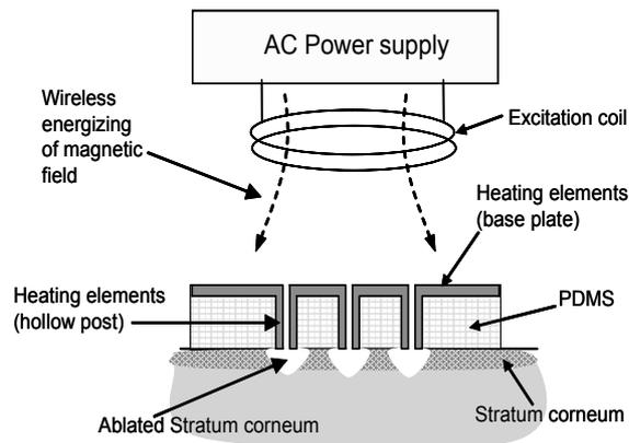
Figure 1. A schematic diagram of wireless inductive heating system for micro-ablation of stratum corneum.
