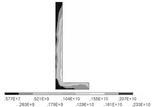
Figure 7. A simulation plot showing induction heating power density at 342kHz (a cross-sectional view,  $W/m^3$ )
