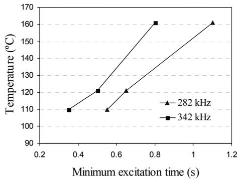
Figure 4. The induction heating characteristics of the hollow post array, type B (in Figure 2b)
