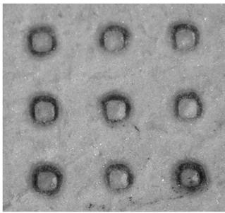
Figure 5. Photograph of the liquid crystal polymer paper (121°C – temperature indicator) after applying induction heating of hollow metallic posts (in Figure 2b)
