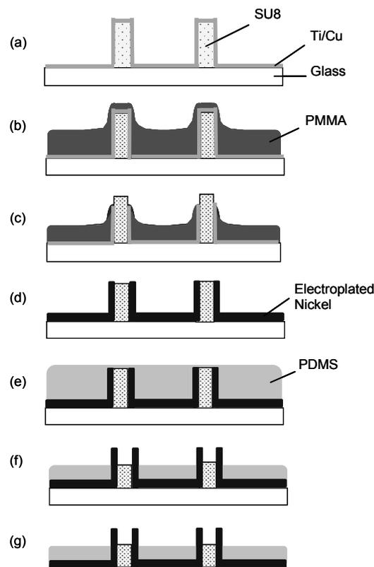
Figure 3. The fabrication process of the micro-heating element (Type B).
