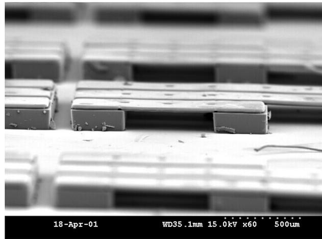
**Figure 4.** Close-up of the SU-8 stand-off that insulates the upper electrode from the silicon substrate. The SU-8 structure is  $125\ \mu\text{m}$  thick and the electroplated NiFe is approximately  $35\ \mu\text{m}$  thick. The thickness of the SU-8 layer allows for a minimum parasitic capacitance and a maximum actuation voltage.
