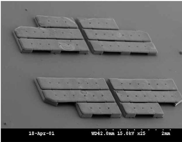
**Figure 2.** Overview of upper NiFe electrodes for silicon oscillator. The uncrosslinked SU-8 has been removed. Multiple electrodes are fabricated so that some may serve as actuators and others as capacitors. The process flow from figure 1 was used in the fabrication.
