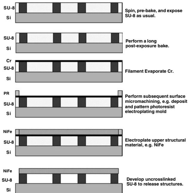
**Figure 1.** General process flow for using uncrosslinked SU-8 as a sacrificial layer.
