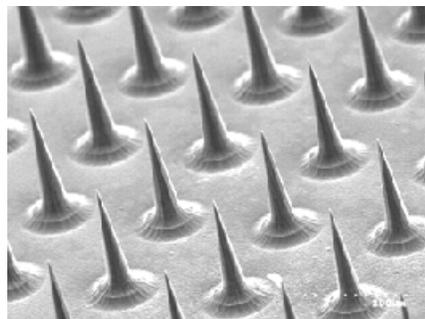
**Figure 2.** PMMA microneedle array before adding electrical functionality.
