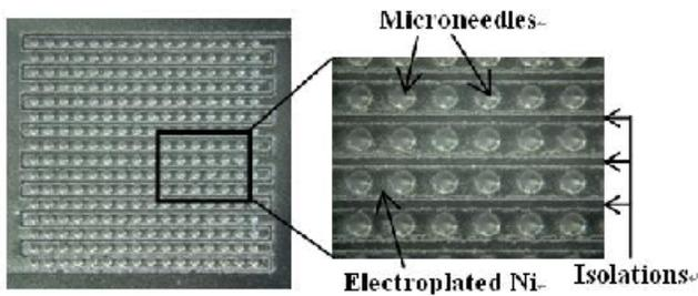
**Figure 3.** Photomicrograph of microneedle electrode device, showing an interdigitated pattern of electrically isolated rows of microneedles.
