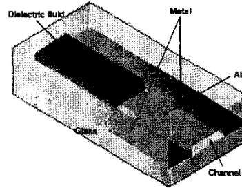
Fig 2. Schematic of a gap capacitor
