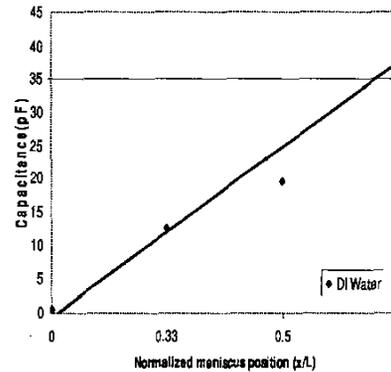
Fig 4. Capacitance according to meniscus position
