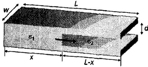
Fig 1. Schematic of the bifluidic capacitance model
