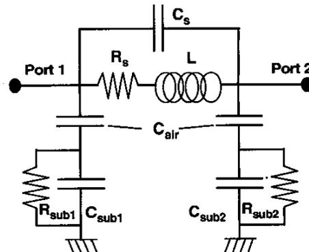
Fig.6. Physical based hybrid model for suspended spiral inductor.
