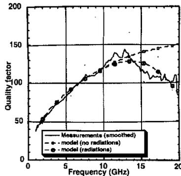
Fig.9. Measured performances and physical based model for 1.5 turns and 350µm diameter suspended inductor.
