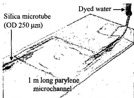
**Figure 5.** Tubing and leakage test.
