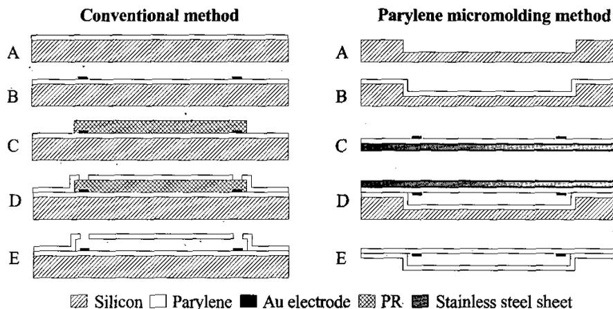
**Figure 1.** Conventional surface micromachining method and new 'parylene micromolding' method of fabricating parylene microchannel (**Surface micromachining method** - A: parylene deposition, B: electrode patterning, C: sacrificial PR patterning, D: parylene deposition and patterning, E: dissolution of PR, **parylene micromolding method** - A: silicon mold fabrication using deep RIE, B: parylene deposition, C: electrode patterning, D: thermal bonding, E: releasing).
