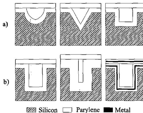
**Figure 2.** Cross-sectional geometries of parylene channels: a) the effect of isotropically and anisotropically etched silicon molds, b) Inner aspect ratio control by varying parylene thickness, and multiple layer channel.
