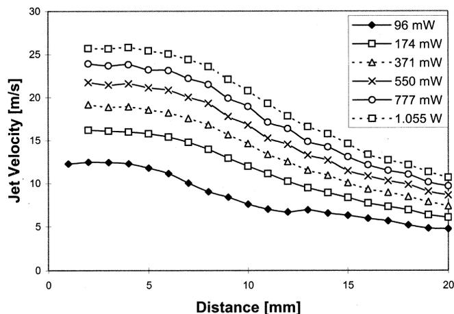
Fig. 10. Center stream jet velocity of the microjet cooling device as a function of the separation distance from the orifice with a variation of the driving power at a fixed resonance frequency.
