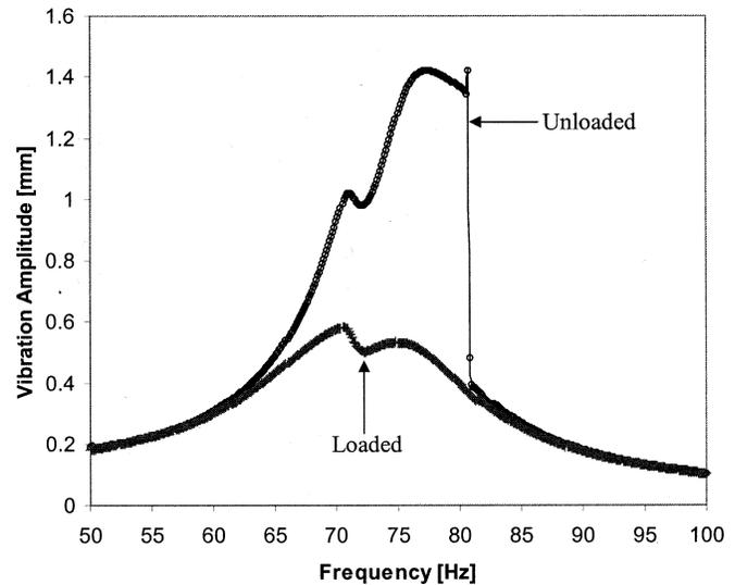
Fig. 3. Vibration amplitude,  $A$ , at the center of the latex membrane-based microjet cooling device as a function of the frequency for a driving voltage of  $V_{ac} = 450$  MV rms; the vibration amplitude is shown for a loaded (with orifice plate) and an unloaded (without an orifice plate) membrane.
