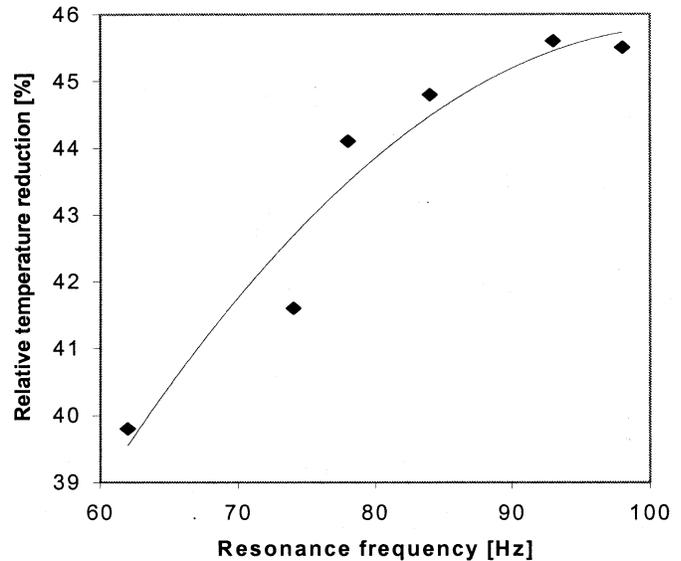
Fig. 7. Cooling performance of the microjet cooling device as a function of resonance frequency. Parameters for microjet cooling device are orifice diameter of  $3/32''$ , orifice to test die spacing of 15 mm, and driving power of 0.55 W.
