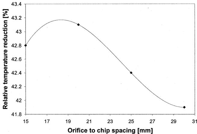
Fig. 6. Cooling performance of the microjet cooling device as a function of spacing from the DIP-28 package (PST-4 thermal test die) to the orifice. Parameters for microjet cooling device are orifice diameter of 2.38 mm, resonance frequency of 80 Hz, and driving power of 0.35 W.
