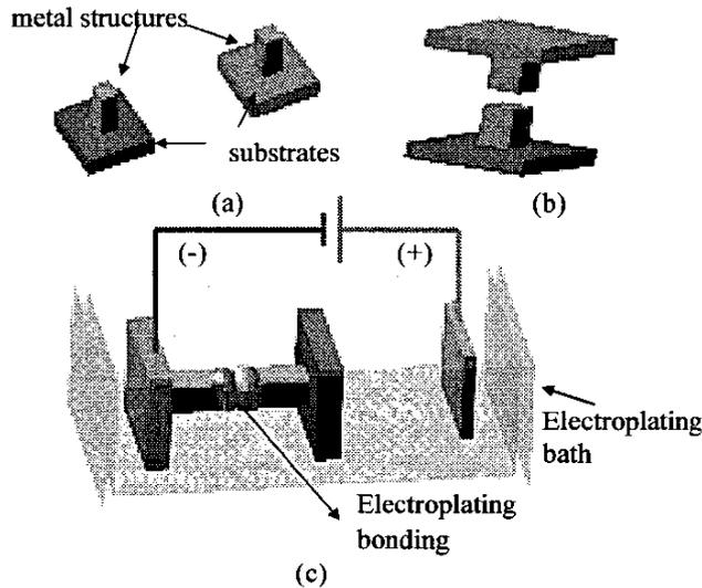
Figure 1. Schematic of electroplating bonding procedure. (a) surface micromachined metal structures (b) structure alignment (c) electroplating bonding in electroplating bath.
