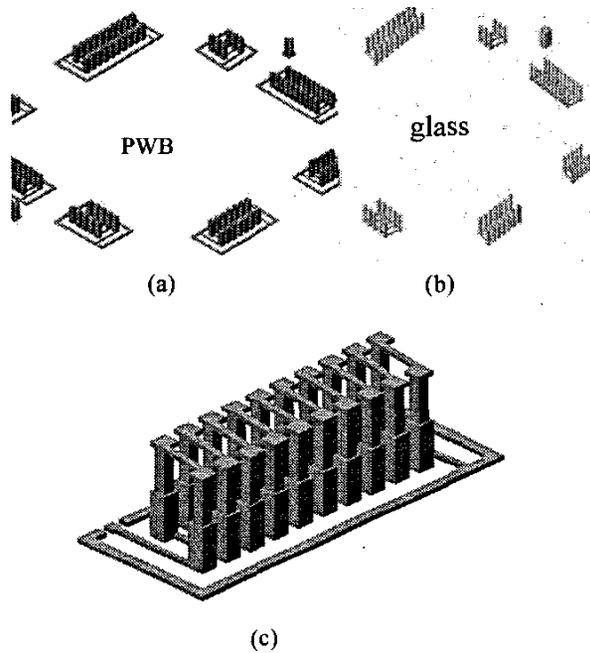
Figure 9. Schematic of micro solenoid inductor. (a) bottom and (b) upper Cu structure before electroplating bonding. (c) electroplating bonding of epoxy-core, micro solenoid inductor.
