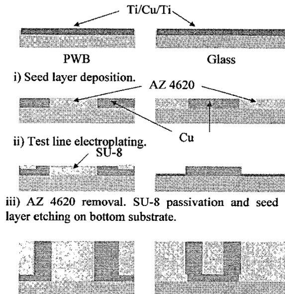
iv) Seed layer deposition on bottom substrate. SU-8 mold and Cu electroplating.
