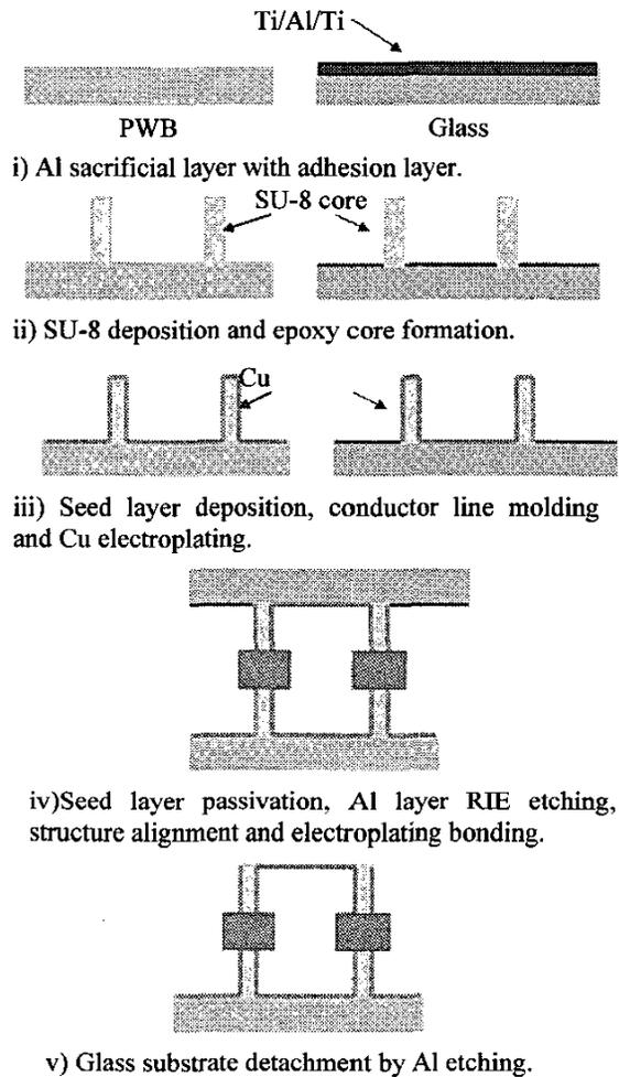
Figure 10. Process schematic of the electroplating bonding epoxy-core inductors.
