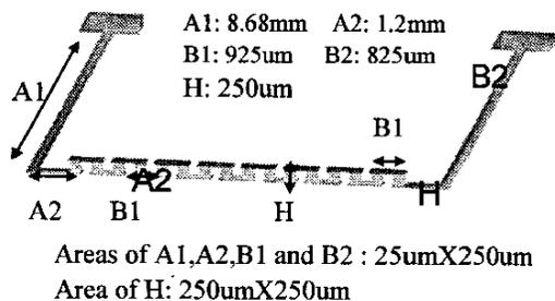
Figure 4. Schematic of the test line.
