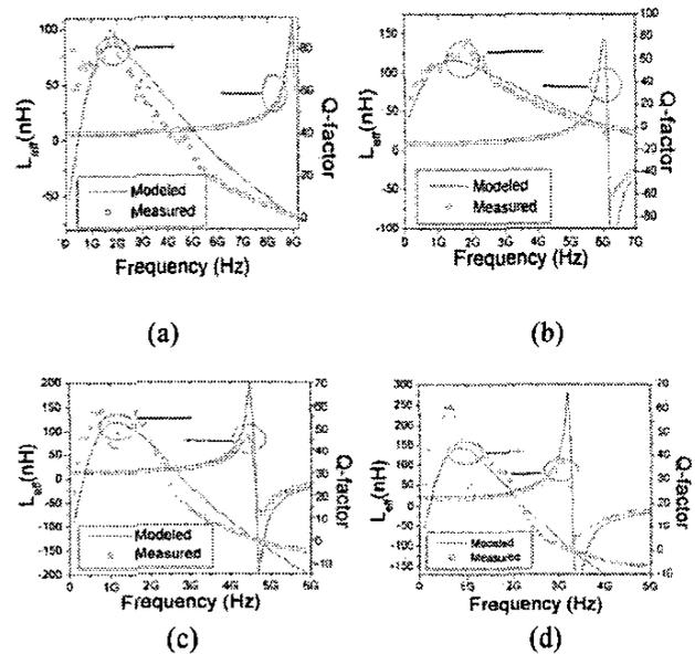
Figure 13. Measured and modeled  $L_{eff}$  and Q of the inductors. From upper (a)3 turn, (b)5 turn, (c) 7turn and (d)10 turn inductor.
