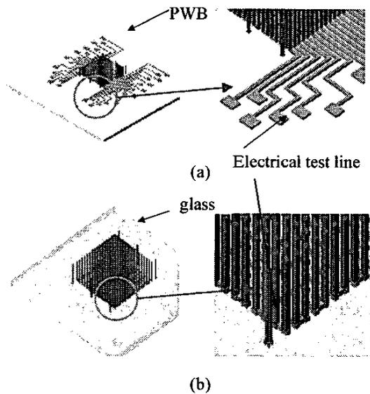
Figure 3. Schematic of electroplating bonding chip interconnects (a) on PWB and (b) on glass substrates.
