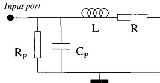
Figure 12. One-port inductor electrical model used for the performance optimization.
