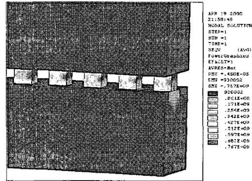
Figure 7. FEM simulation of chip interconnects.
