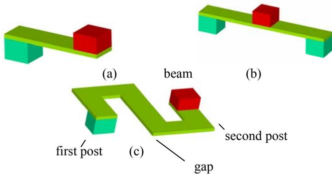
**Figure 1:** Schematic of surface micromachined interconnects. (a) Step type (b) Bridge type (c) Semi-spiral type.
