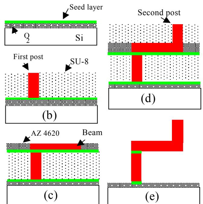
**Figure 2:** Fabrication process of flexible interconnect.
