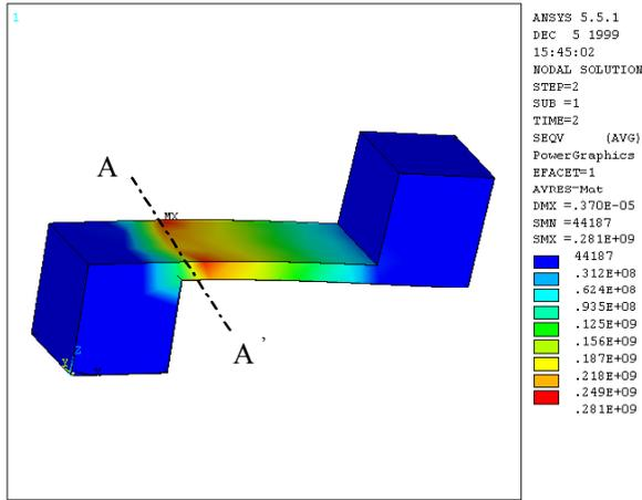
Figure 5: Stress simulation of stair interconnects with 0.02mN applied load.
