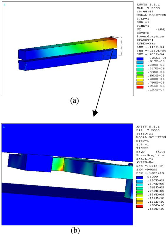
**Figure 9:** Thermal expansion and resultant stress for 16 semi-spiral interconnects under 100 degree C temperature variance.
