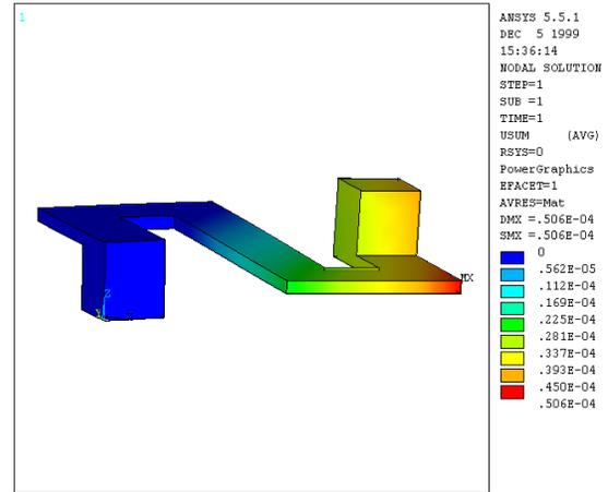
Figure 7: ANSYS simulation for semi-spiral type interconnects with 0.025mN load.
