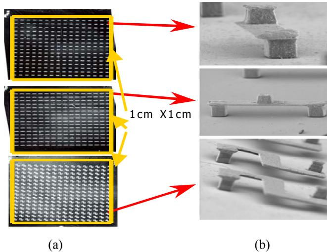
**Figure 3:** Photomicrograph (a) and scanning electron micrograph (b) of fabricated surface micromachined flexible interconnect structures.
