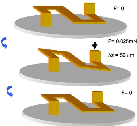
Figure 6: Semi-spiral type interconnect acting like a spring under 0.02mN applied load.
