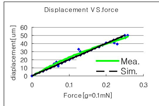
Figure 8: Comparison of measurement and simulation data for displacement of semi-spiral type structure.
