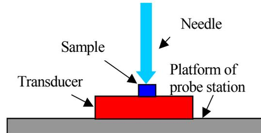
**Figure 4:** The measurement system for mechanical deflection of the interconnects.
