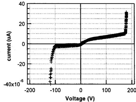
**Figure 3:** I-V curve for a single thermomigrated npn junction. The breakdown voltage is at -110V and +170V for reverse and forward biases, respectively.
