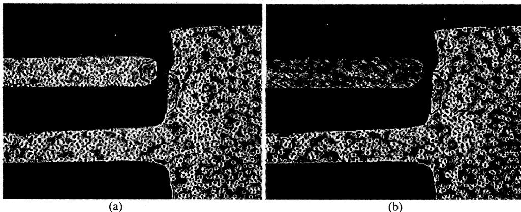
**Figure 8:** Photomicrographs of the junction isolated demonstration actuator with and without an excitation voltage. In (a), no excitation is applied. In (b), the excitation voltage is 162Vpp with a 84V offset at 60Hz. The finger displacement is approximately 10 $\mu$ m, resulting in a blurring of the rotor comb shown in (b).
