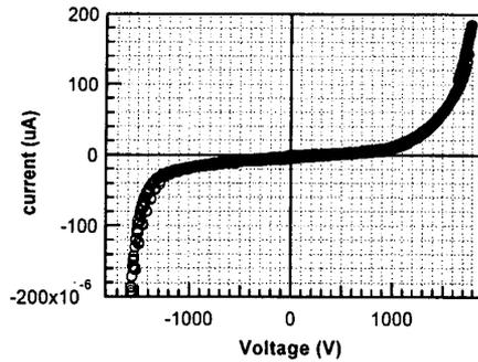
**Figure 5:** *I-V curve for 12 thermomigrated npn junctions. For 12 npn junctions, the breakdown voltages sum, with a resultant overall breakdown voltage of -1550V and +1450 V.*
